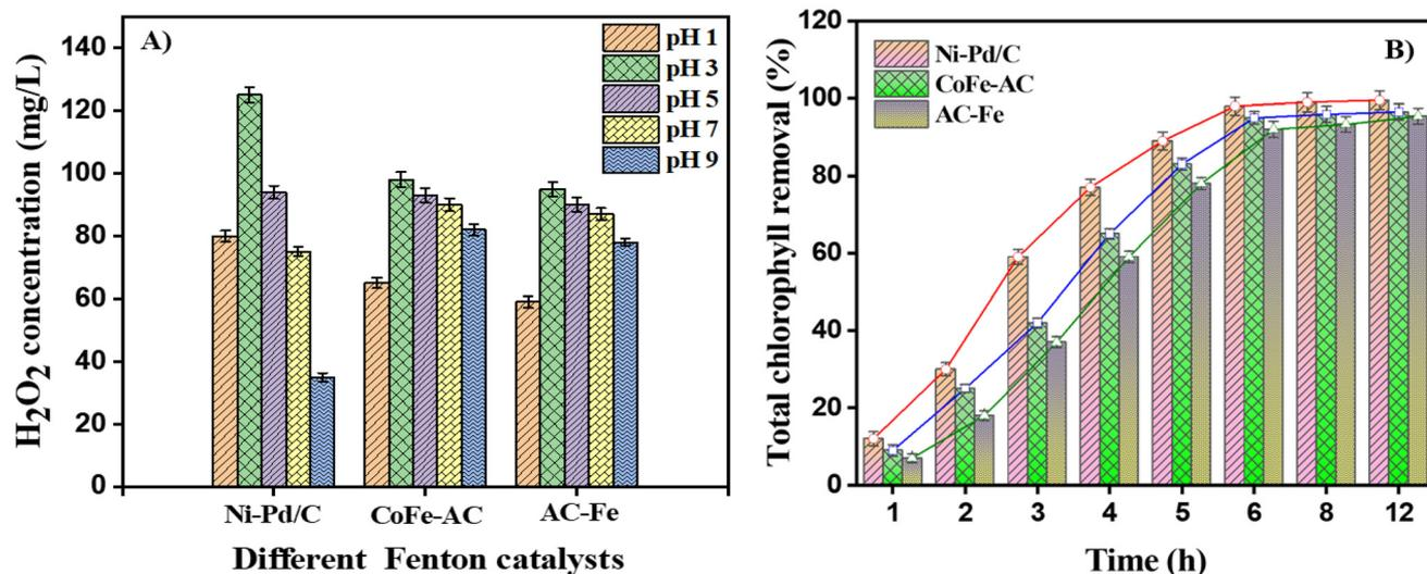
Fig. 7 (A) Variation of different H<sub>2</sub>O<sub>2</sub> concentrations produced by employing different catalysts under the pH range from 1.0 to 9.0; (B) total chlorophyll removal (%) during the different time intervals.
