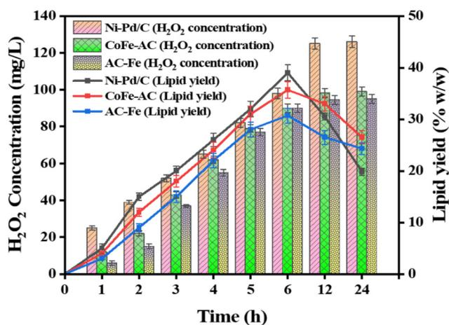
Fig. 8 Algal lipid yield obtained under different H<sub>2</sub>O<sub>2</sub> concentrations produced by Ni-Pd/C, CoFe-AC, and AC-Fe catalysts.
