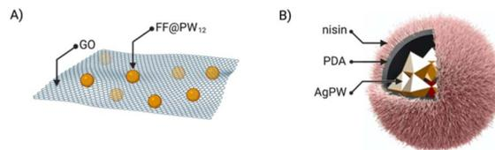
Fig. 7 Ternary composites of ionic POM-peptide hybrids: (A) FF@PW<sub>12</sub>@GO and (B) AgPW@PDA@nisin, adapted from ref. 52 with permission, Elsevier, copyright 2020.
