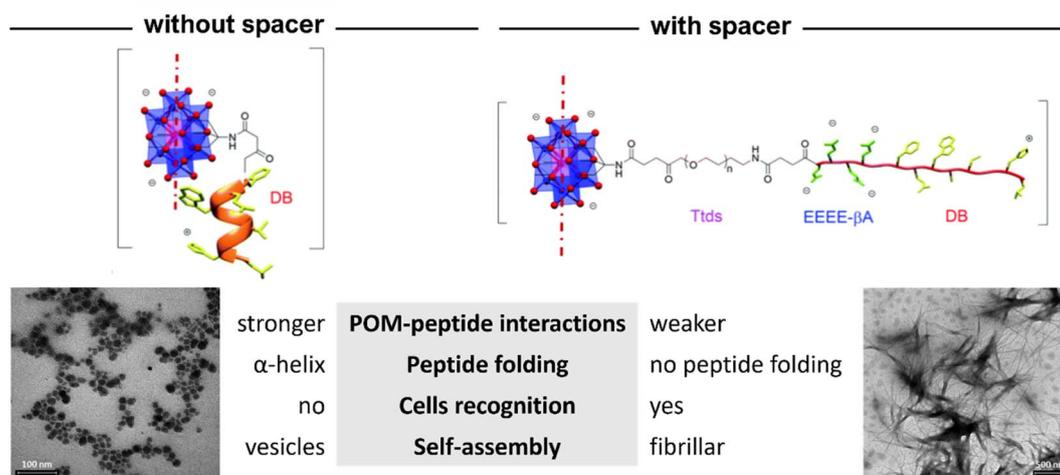
Fig. 15 Structural differences between the hybrids of POM–(demobensin-1)<sub>2</sub> without and with spacer between the Mn–Anderson–Evans POM and the peptide. Adapted with permission from ref. 70, Royal Society of Chemistry, copyright 2021.
