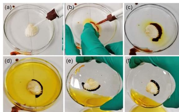
Fig. 12 Photographs showing the curing and adhesion efficacy of the peptide/POM coacervates system based on {BW<sub>12</sub>} and {HPMo<sub>10</sub>V<sub>2</sub>} POMs. (a) A shell is immersed in water in a watch glass and (b) the coacervates are injected simultaneously. (c) and (d) Crosslinking of the shell takes place spontaneously. (e) and (f) Tilting tests show the effectiveness of the adhesion. Reprinted with permission from ref. 76. Copyright 2021 American Chemical Society.
