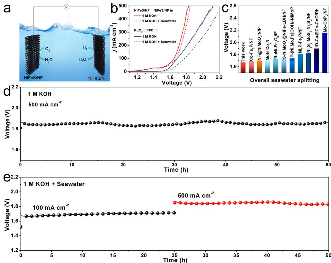
Fig. 4 (a) A schematic illustration of an overall water splitting electrolyzer using NiFeS/NF as both anode and cathode. (b) The overall water/seawater splitting performance of NiFeS/NF||NiFeS/NF and the RuO<sub>2</sub>||Pt/C pairs in 1 M KOH and 1 M KOH + Seawater. (c) Comparison of overpotentials at 100 mA cm<sup>-2</sup> for NiFeS/NF with other bifunctional electrocatalysts. Chronopotentiometry curves of the NiFeS/NF||NiFeS/NF pair in (d) 1 M KOH, and (e) 1 M KOH + Seawater electrolyte.
