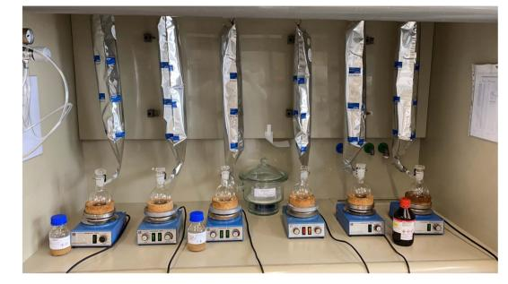
Fig. 1 Silylation work station under argon protection using filled gas bags.
