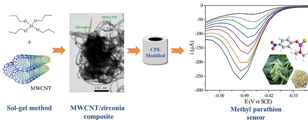
Fig. 6 Scheme of preparation for the MWCNT/ZrO<sub>2</sub>/CPE electrochemical sensor and electrochemical detection of methyl parathion. Reproduced from ref. 101 with permission from Elsevier, copyright 2020.
