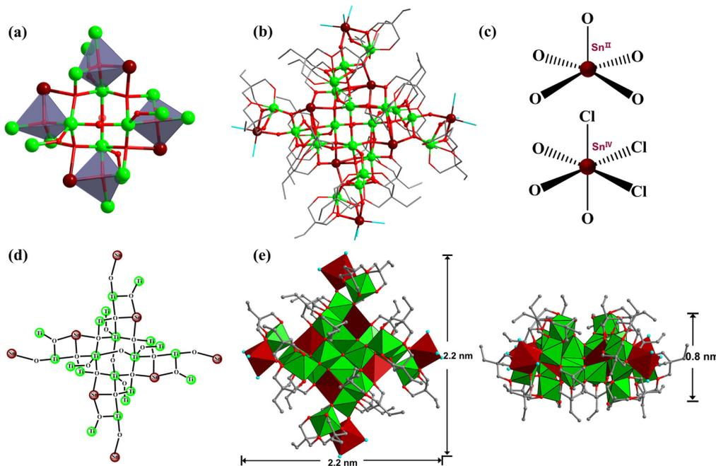
**Fig. 5** (a) Multifaceted view of the  $\text{Sn}_4\text{Ti}_{16}$  internal inorganic core in **TOC-58**. (b) The cluster structure of **TOC-58**. (c) Coordination spheres of the Sn atoms in **TOC-58**. (d) Connection diagram of Ti and Sn atoms through bridging an O atom in **TOC-58**. (e) Polyhedral representations of the  $\text{Sn}_8\text{Ti}_{20}$  core of **TOC-58**.
