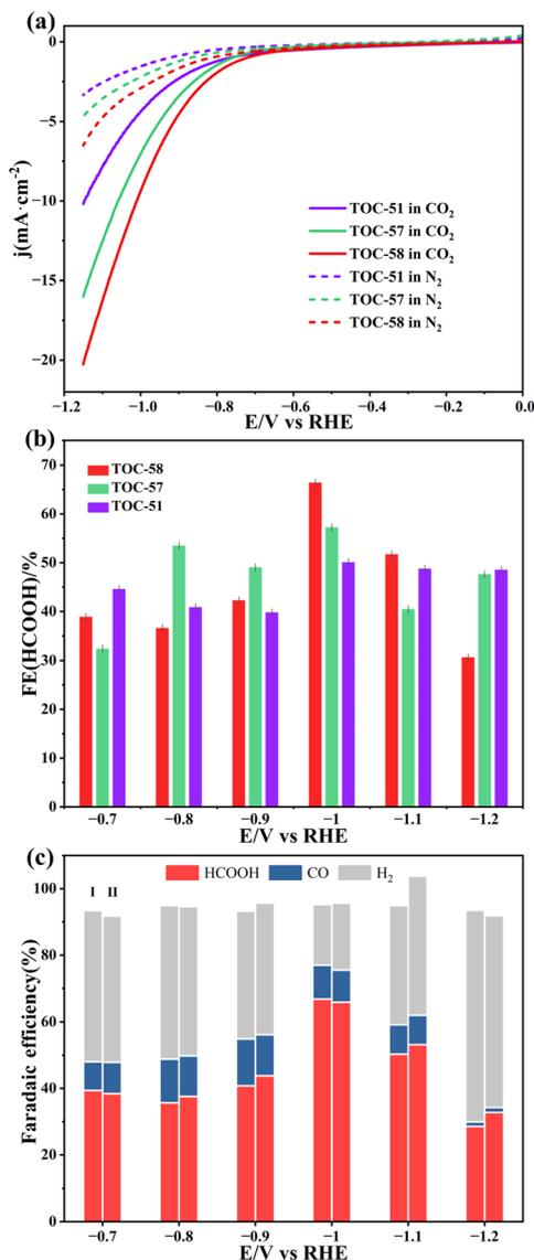
**Fig. 6** (a) LSV profiles of TOC-51-, TOC-57- and TOC-58-decorated electrodes in N<sub>2</sub>- or CO<sub>2</sub>-saturated 0.5 M KHCO<sub>3</sub> solution. (b) Comparative FEs of formates for TOC-51-, TOC-57- and TOC-58-derived electrodes at various potentials. (c) Faradaic efficiencies for formate, H<sub>2</sub> and CO at different potentials of the TOC-58-decorated electrode, showing the results of two different experiments (I and II).
