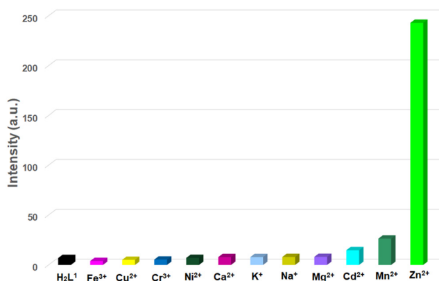
Fig. 12 Relative fluorescence intensity change profile of H_2L^1 in the presence of various cations ( 10^{-2} M) at room temperature (excitation at 446 nm).
