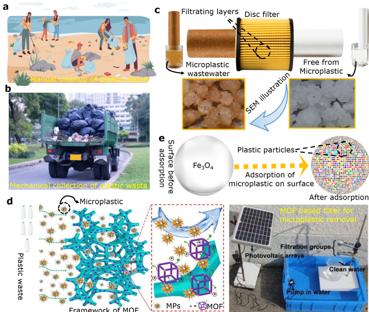
Fig. 2 Manual cleanup efforts for plastic removal near a river area (a). Adapted from ref. 57 Copyright 2021, Springer. Mechanical collection of plastic (b). Adapted from ref. 59 Copyright 2017, Sage. A setup of a disc filter for MP removal in wastewater (c). Adapted from ref. 65 Copyright 2019, MDPI. Zirconium MOF based filter and automatic filtration system for MP removal (d). Adapted from ref. 66 Copyright 2020, the Royal Society of Chemistry. Surface adsorption of plastics on \text{Fe}_3\text{O}_4 (e). Adapted from ref. 67 Copyright 2022, Elsevier.
