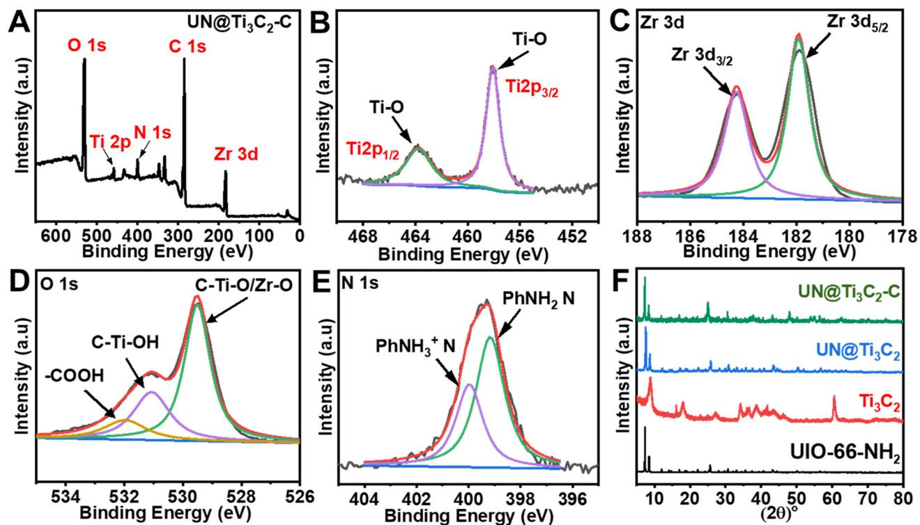
Fig. 3 (A) XPS wide-scan survey spectrum of 50% UN@Ti<sub>3</sub>C<sub>2</sub>-C. (B) Ti 2p. (C) Zr 3d. (D) O 1s. (E) N 1s. (F) XRD patterns of the samples UIO-66-NH<sub>2</sub>, Ti<sub>3</sub>C<sub>2</sub>, UN@Ti<sub>3</sub>C<sub>2</sub>, and UN@Ti<sub>3</sub>C<sub>2</sub>-C.
