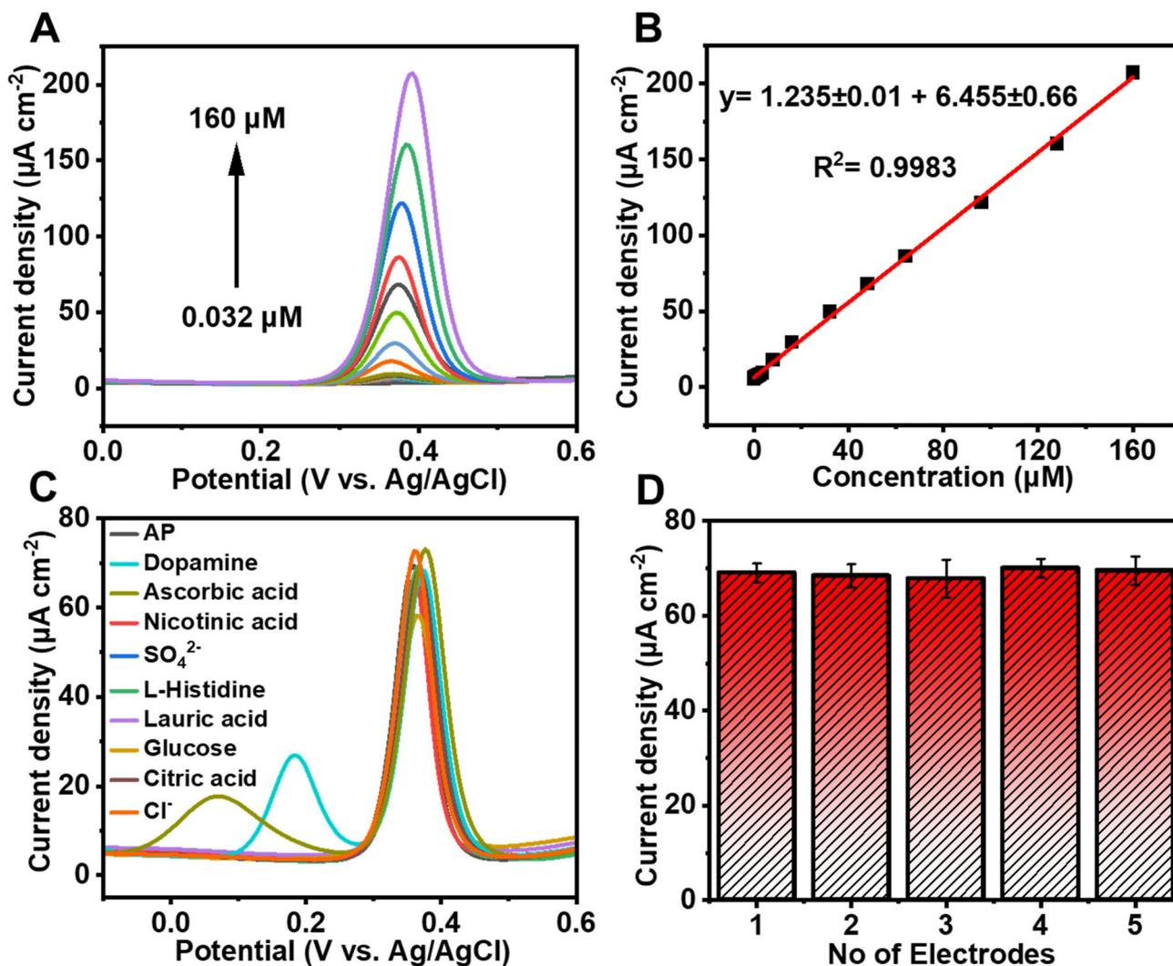
Fig. 5 (A) DPV curves of UN@TT-C/GCE with different AP concentrations from 0.032 to 160  $\mu\text{M}$  in 0.1 M PBS with pH 7.0. (B) Current density ( $\mu\text{A cm}^{-2}$ ) vs. concentration ( $\mu\text{M}$ ) linear calibration plot of AP. (C) DPV of 48  $\mu\text{M}$  AP in 0.1 M PBS (pH = 7.0) using 50% UN@Ti<sub>3</sub>C<sub>2</sub>-C/GCE with 10-time dosage of the different interference species. (D) Reproducibility graph of five electrodes.
