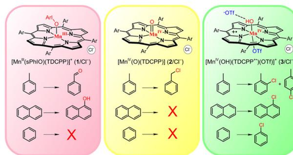
**Scheme 1** Reactions of Mn-porphyrin intermediates with aromatic compounds.
