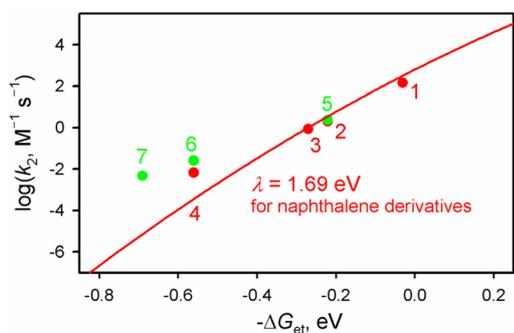
**Fig. 4** Plot of  $\log k_2$  for the oxidation of different substrates [(1) 1-Me-naphthalene, (2) naphthalene, (3) 1-Br-naphthalene, (4) 1-NO<sub>2</sub>-naphthalene, (5) anisole, (6) toluene, and (7) benzene] vs. the driving force of electron transfer [ $-\Delta G_{\text{et}}$ ; eqn (2)] by  $3/\text{Cl}^-$  in  $\text{CH}_2\text{Cl}_2$  at  $-10$  °C.
