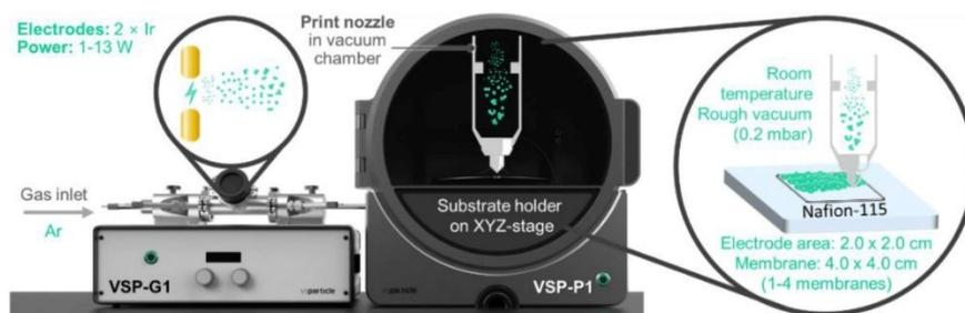
Figure 5. Schematic of the VSParticle nanoparticle printing technology. A certain wattage is applied to metal electrodes which causes the metal to ablate and particles to detach. The particles agglomerate to form nanoparticles as they are carried by inert Ar to a vacuum chamber where they are printed *via* nozzle onto a substrate of choice held by a XYZ-stage. Reproduced with permission from Reference 110. Copyright 2022 MDPI.
