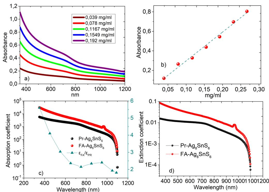
**Fig. 5** (a) UV-vis spectra and the corresponding calibration curves (b). Absorption coefficient ( $\epsilon$  in M<sup>-1</sup> cm<sup>-1</sup>) (c) and extinction coefficient ( $k$  in M<sup>-1</sup>) (d) values in the range 380–1200 nm for the Pr–Ag<sub>8</sub>SnS<sub>6</sub> and FA–Ag<sub>8</sub>SnS<sub>6</sub>. The ratio between  $\epsilon_{FA}/\epsilon_{PR}$  can be seen in Fig. 5c.
