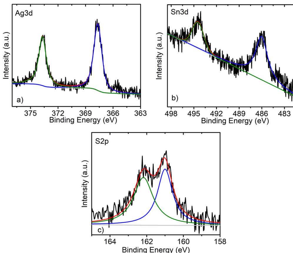
Fig. 3 XPS spectra of the (a) Ag 3d, (b) Sn 3d and (c) S 2p peaks recorded from the sample Pr-Ag<sub>8</sub>SnS<sub>6</sub>.
