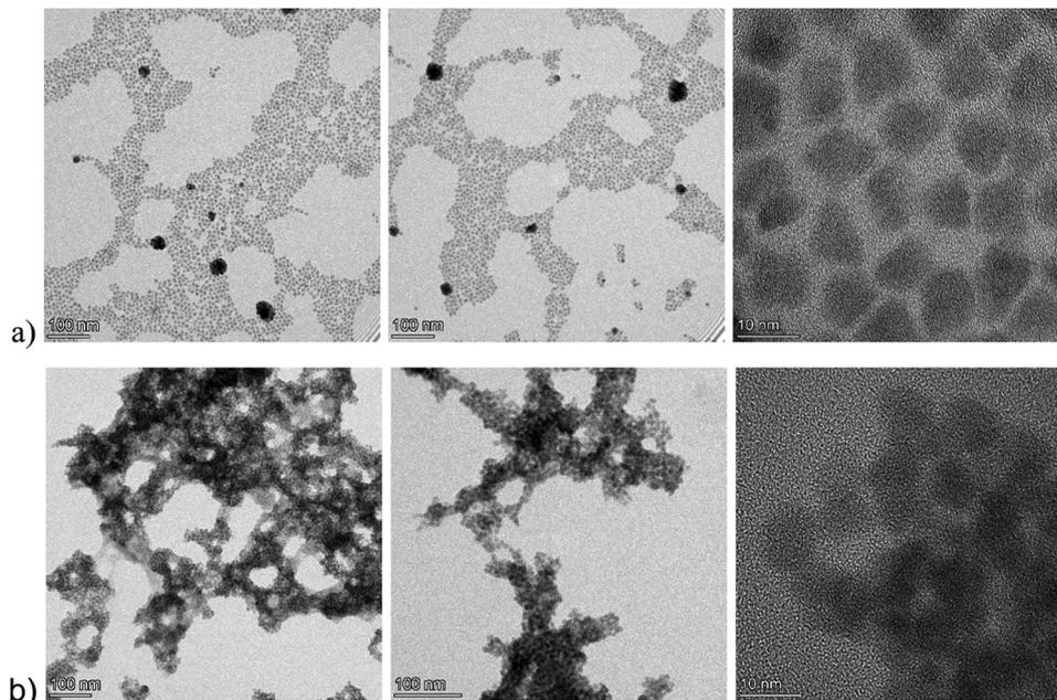
Fig. 1 Representative TEM bright-field images of the pristine, Pr-Ag<sub>8</sub>SnS<sub>6</sub>, particles (a) and the functionalized FA-Ag<sub>8</sub>SnS<sub>6</sub> (b). The particles appearing with high contrast are silver-rich phases that are formed under the influence of the electron beam.
