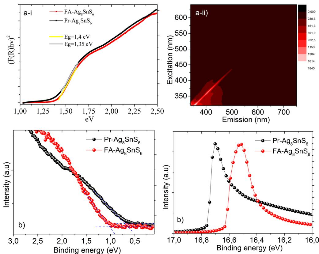
Fig. 6 (a) (i) Tauc plots of Pr-Ag<sub>8</sub>SnS<sub>6</sub> and FA-Ag<sub>8</sub>SnS<sub>6</sub> and the calculated band gap. (ii) Excitation dependent photoluminescence maps. (b) UPS spectra of Pr-Ag<sub>8</sub>SnS<sub>6</sub> and FA-Ag<sub>8</sub>SnS<sub>6</sub> for the calculation of Fermi level (left) and valence band maximum (right).
