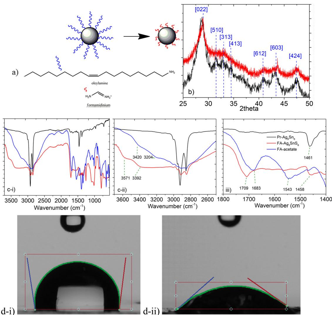
Fig. 4 (a) Schematic representation of the exchange of oleylamine with the formamidinium (b) XRD patterns of the Pr- $\text{Ag}_8\text{SnS}_6$  and FA- $\text{Ag}_8\text{SnS}_6$  samples. (c) FTIR spectra in three different areas (d) contact angle measurements for Pr- $\text{Ag}_8\text{SnS}_6$  (i) and FA- $\text{Ag}_8\text{SnS}_6$  (ii).
