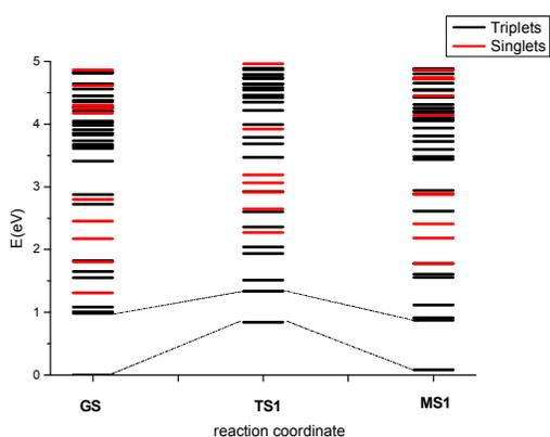
**Figure 7** Energy profiles for the GS->MS1 transition in the ground and photoexcited states. Triplet and singlet states are indicated by black and red lines, respectively. The excited states were computed at the TD-DFT/M06/LANL2DZ/6-311++G(d,p) level of theory with water as a continuum.
