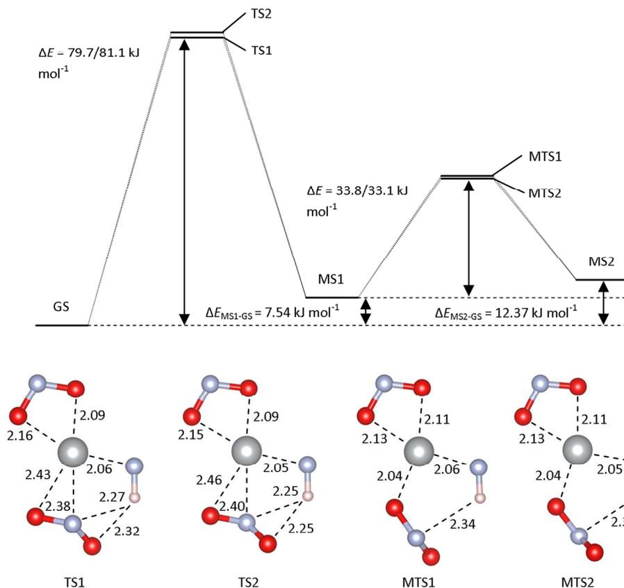
**Figure 4** Schematic of the isomerisation pathways in  $[\text{Ni}(\text{Et}_4\text{dien})(\eta^2\text{-O,ON})(\eta^1\text{-NO}_2)]$ , modelled using the M06 functional and the LANL2DZ/6-311++G(d,p) basis set, and with water as a continuum. The energy profile illustrates the relative energies of the GS, MS1 and MS2 isomers, and the transition states connecting them, while the four models show the optimised geometries of the four transition states.
