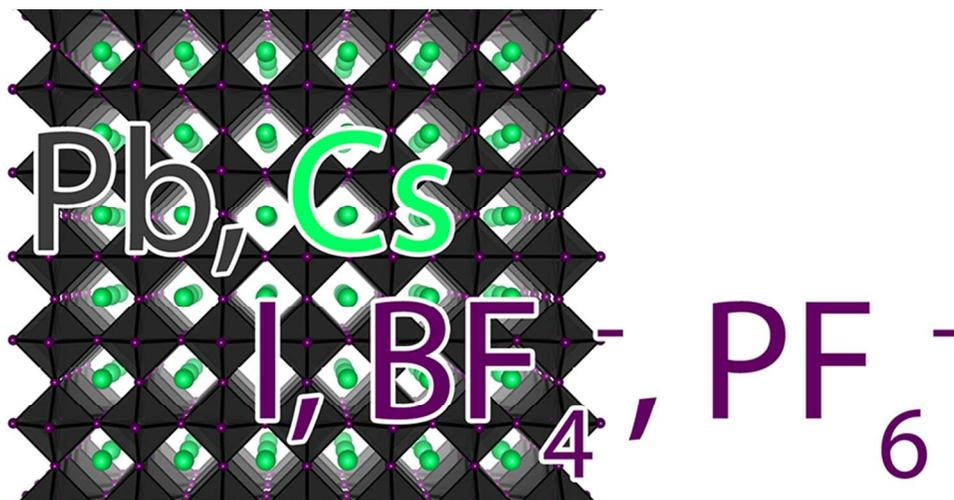
The incorporation of tetrafluoroborate and hexafluorophosphate in halide perovskites are found to result in substantial band gap widening.
