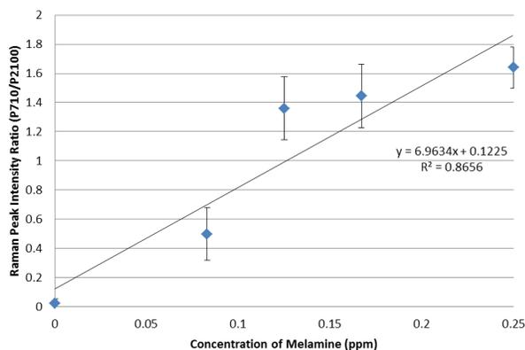
**Fig. 4.** A concentration standard curve showing the effect of melamine (M) concentration on a Raman peak intensity ratio (P710/P2100) in the presence of acetoguanamine (A) [M+A = 0.25 ppm for all samples].
