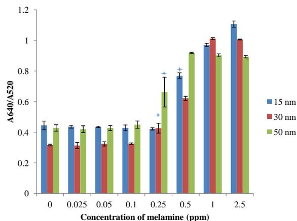
**Fig. 1.** The absorption ratio ( $A_{640}/A_{520}$ ) versus different concentrations of melamine in water (0 ppm, 0.025 ppm, 0.05 ppm, 0.1 ppm, 0.25 ppm, 0.5 ppm, 1 ppm and 2.5 ppm) when the diameters of Au NPs were 15 nm, 30 nm and 50 nm, respectively. The limit of detection (LOD) of melamine for 15 nm, 30 nm and 50 nm Au NPs was 0.5 ppm, 0.25 ppm, and 0.25 ppm respectively, as indicated by a blue star on the graph (based on T-test).
