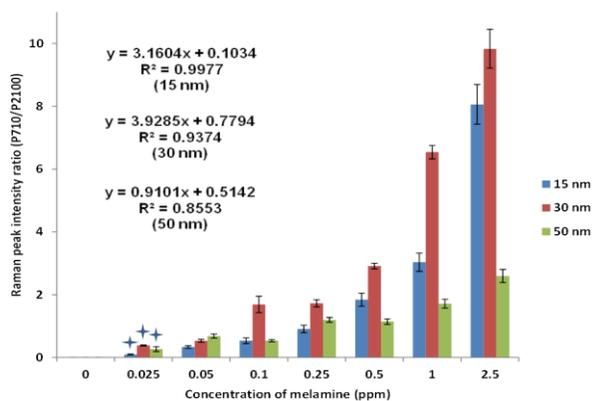
**Fig. 2.** The SERS peak intensity ratio of the melamine peak to Au NP peak (P710/P2100) versus different concentrations of melamine in water (0 ppm, 0.025 ppm, 0.05 ppm, 0.1 ppm, 0.25 ppm, 0.5 ppm, 1 ppm and 2.5 ppm) when the diameters of Au NPs were 15 nm, 30 nm and 50 nm respectively. The limits of detection (LODs) for 15 nm, 30 nm and 50 nm Au NPs were all 0.025 ppm, as indicated by a blue star (based on T-test).
