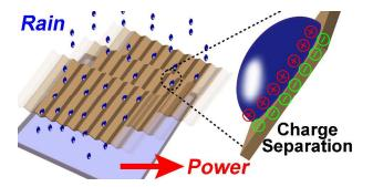
When water droplets (e.g., from rain) flow down a solid surface due to gravity, they can generate power.
