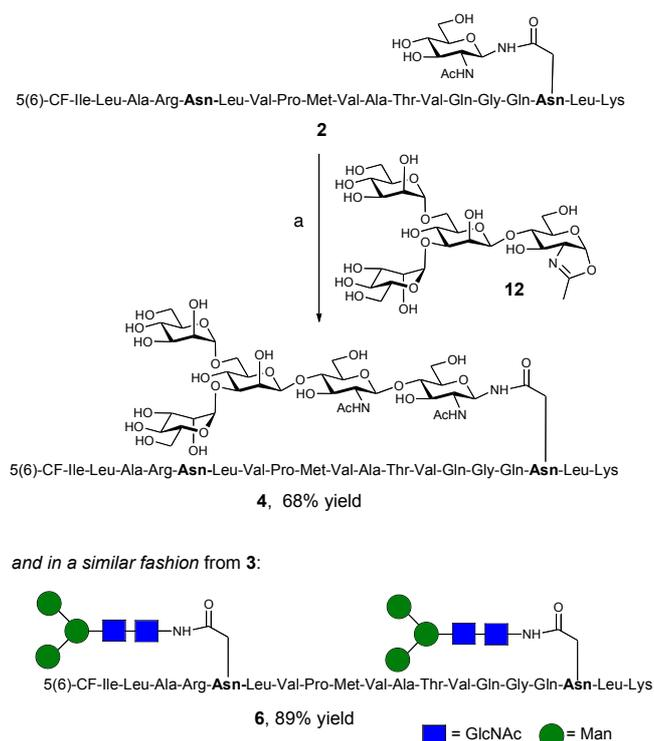
**Scheme 2.** Reagents and conditions: (a) oxazoline **12**, Endo A E173H, sodium phosphate buffer (100 mM, pH 6.5), 23 °C, 7 h.
