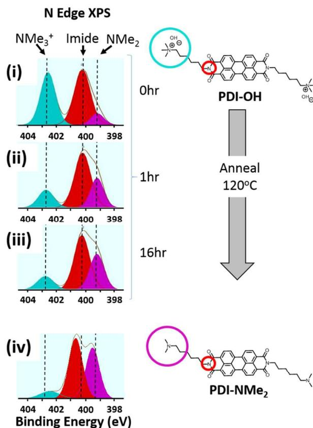
**Figure 2.** Conversion of NMe<sub>3</sub><sup>+</sup> to NMe<sub>2</sub> in PDI-OH proceeds upon thin film annealing at 120 °C (i-o hrs, ii-1 hr, iii-16 hrs) as observed via XPS (N 1s spectra). As expected, after extended annealing, the
