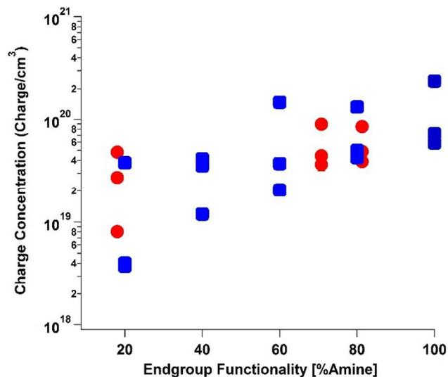
**Figure 3.** Electron paramagnetic resonance (EPR). Quantitative measurements of charge carrier concentration in PDI samples were done in triplicate for all samples: (1) PDI-NMe<sub>2</sub>/PDI-C6 composites with varying PDI-NMe<sub>2</sub> content (blue squares), (2) annealed PDI-
