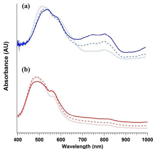
**Figure 4.** Evolution PDI thin film optical absorption spectra with anneal time: 0 min (light dotted line), 20 min (dashed line), and 1 hr (dark solid line) for (a) PDI-OH and (b) PDI-NMe<sub>2</sub>.
