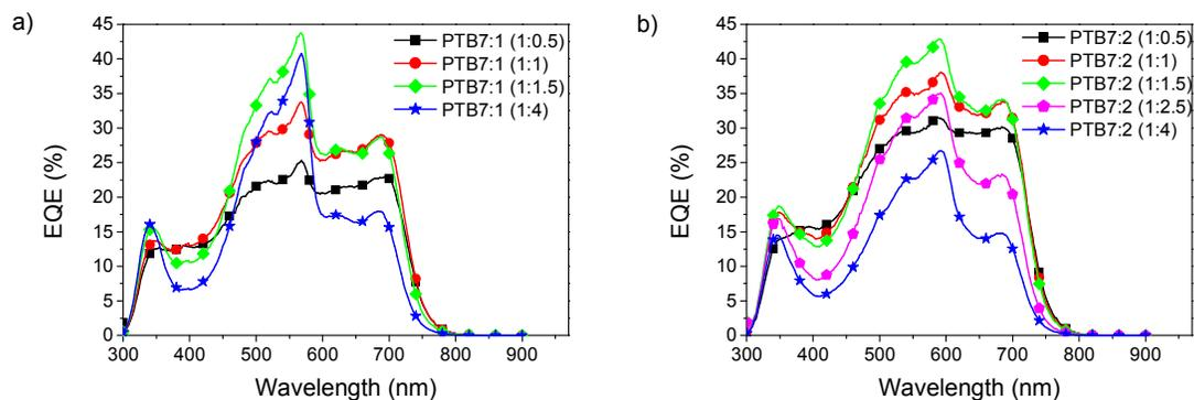
**Fig. 6** Influence of the blend ratio of PTB7:1 (a) and PTB7:2 (b).
