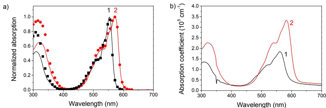
**Fig. 2** a) Absorption of **1** and **2** in chlorobenzene solution (solid lines) and fluorescence excitation spectra (symbols) showing complete transparency in the region of 400 to 425 nm. b) Absorption spectra of films of **1** and **2** spin coated from chlorobenzene.
