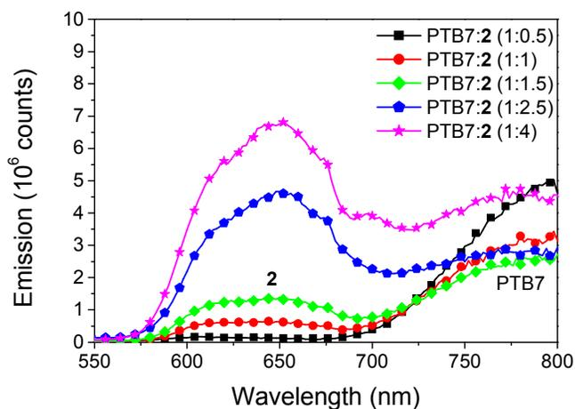
**Fig. 9** Fluorescence emission spectra of PTB7:2 for varying blend ratio. The excitation wavelength was 280 nm. The emission at 650 originates from compound **2** and the emission at 800 nm from PTB7.
