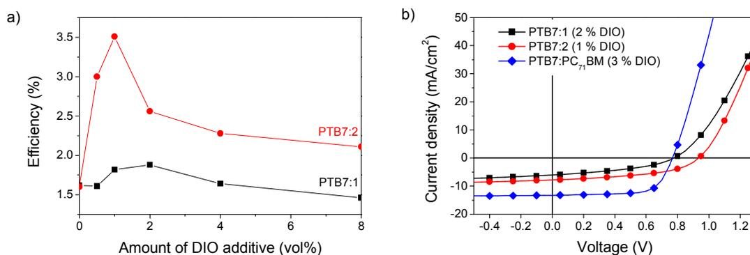
**Fig. 7** a) Power conversion efficiency of PTB7:1 and PTB7:2 as a function of the amount of solvent additive DIO. b) JV-curves of optimized solar cells in comparison to PTB7:PC<sub>71</sub>BM.
