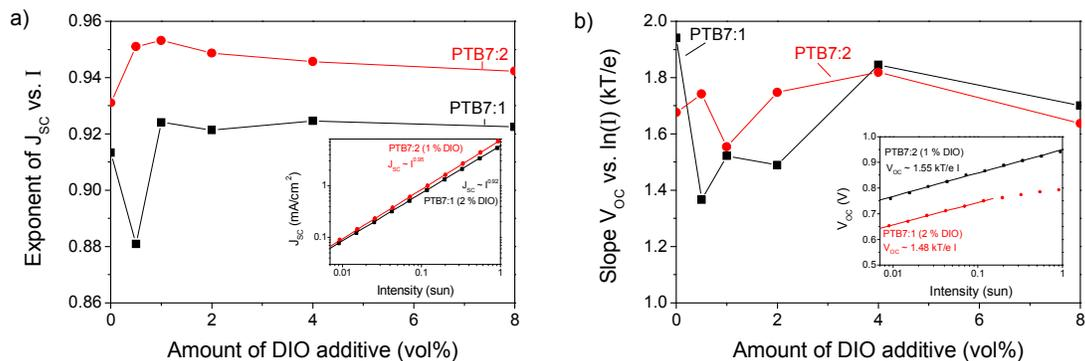
**Fig. 8** a) The exponent of the short circuit density vs. light intensity ( $I$ ) as a function of content of DIO. The inset shows an example at the optimized conditions. b) Slope of the open circuit voltage as a function of content of DIO. The inset shows an example at the optimized conditions.
