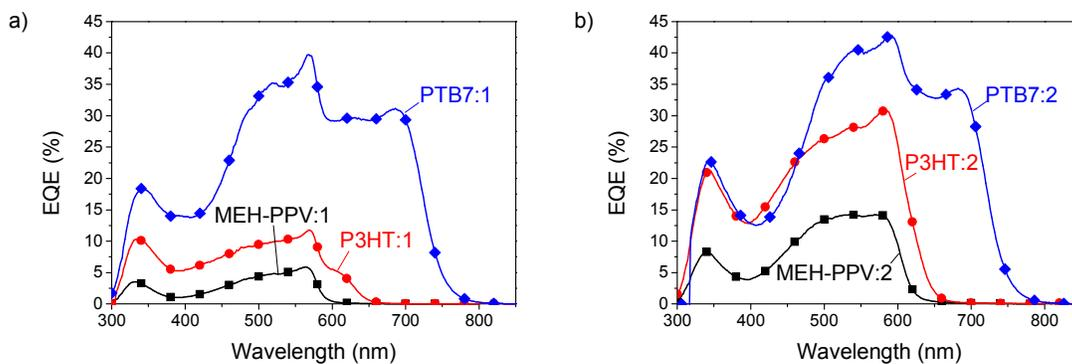
**Fig. 4** EQE spectra of MEH-PPV (squares), P3HT (circles) and PTB7 (diamonds) blended with compound **1** (a) and compound **2** (b).
