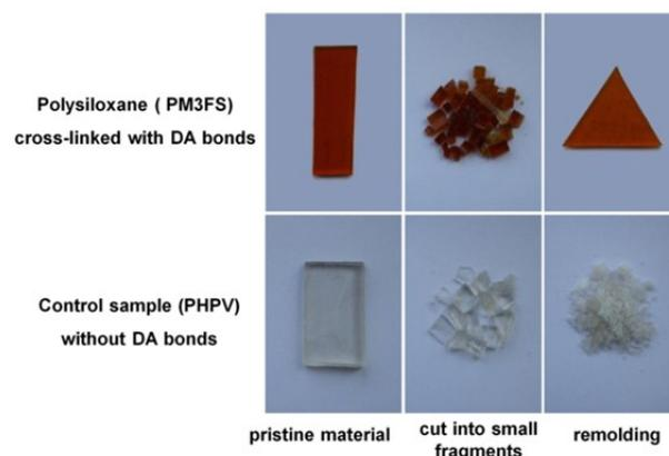
**Fig. 3** The remoldability of the cross-linked polymers PM3FS and PHPV.
