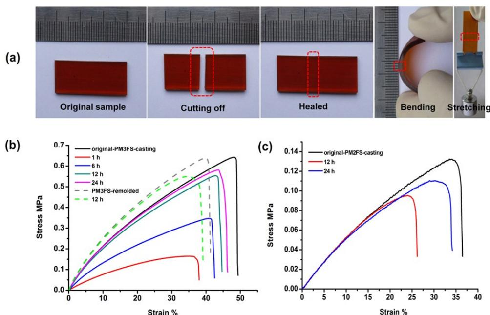
**Fig. 4** The self-healing properties of the PMFS polymers: (a) the healed PM3FS sample can be bent or stretched, (b) stress–strain curves of the PM3FS prepared through casting method (solid lines) and compression molding method (dotted lines) healed for different times, (c) stress–strain curves of the PM2FS prepared through casting method healed for 12 and 24 h.
