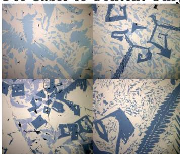
Optical images of the surface patterns formed by hexaboride ( $\text{MB}_6$ ) and dodecaboride ( $\text{MB}_{12}$ ) phases.
