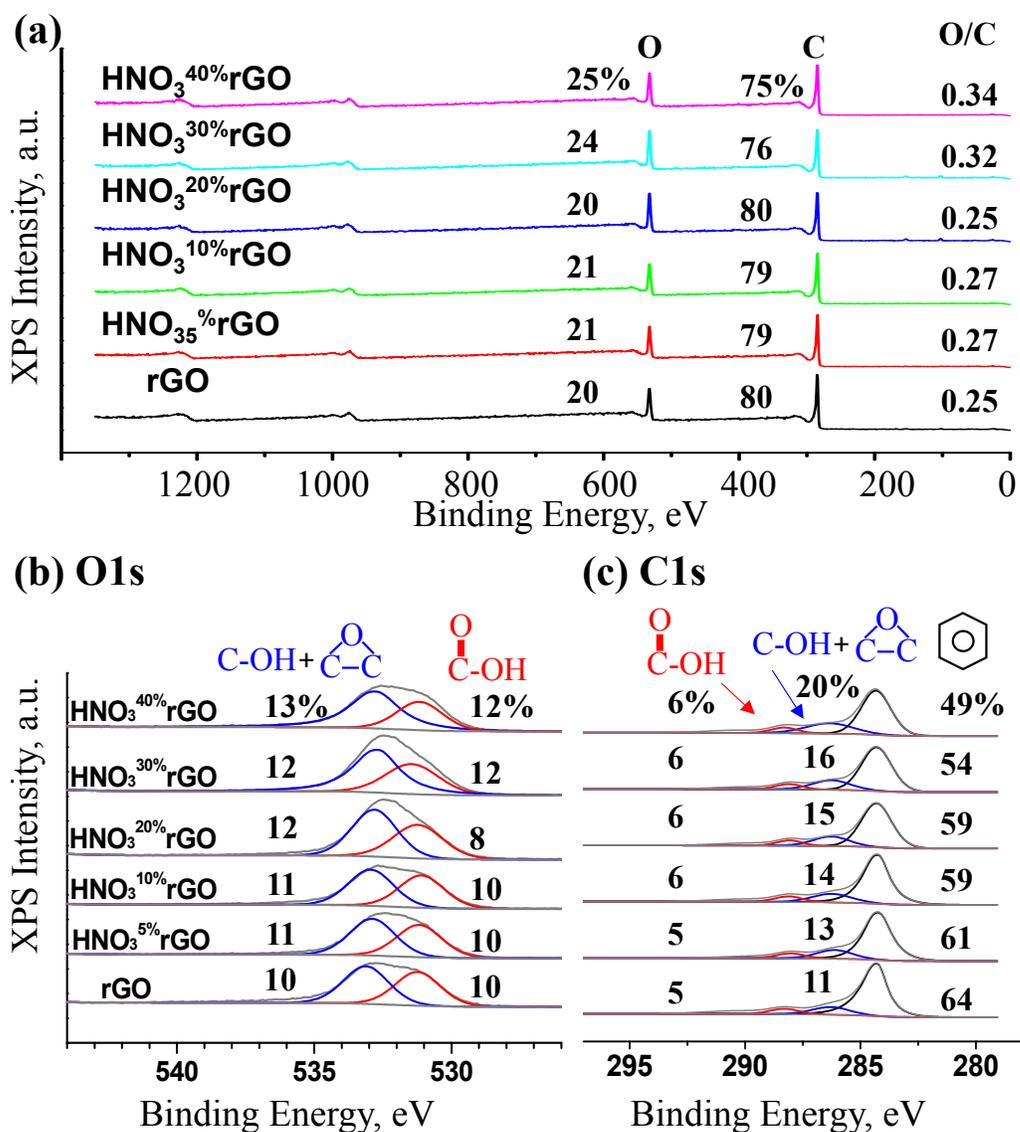
**Figure 5.** XPS spectra of the initial and  $\text{HNO}_3$ -treated rGO materials.
