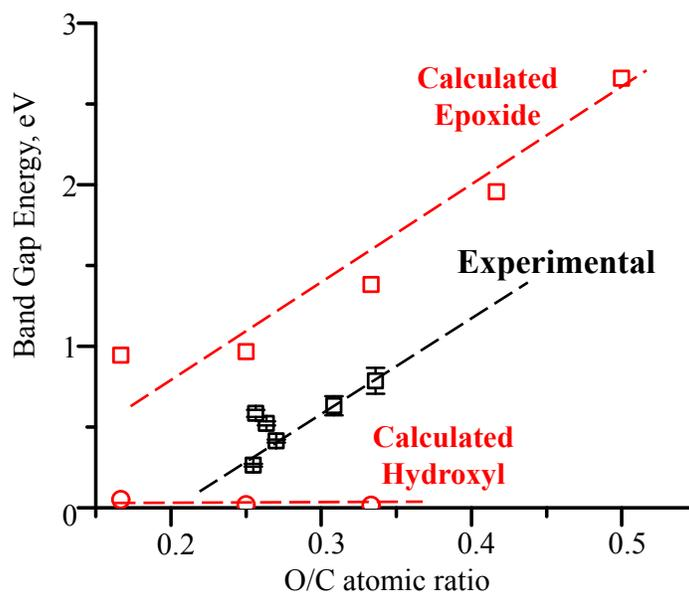
**Figure 9.** Experimental and computational dependencies of the rGO band gap energy on the extent of oxidation.
