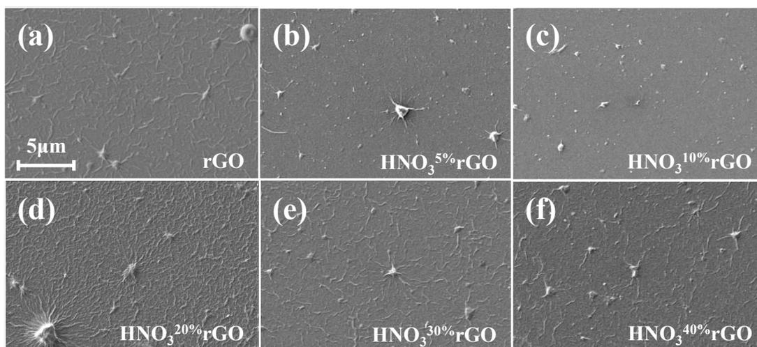
**Figure 2.** SEM images of (a) rGO and (b-f)  $\text{HNO}_3$ -treated rGO films on Si wafers.
