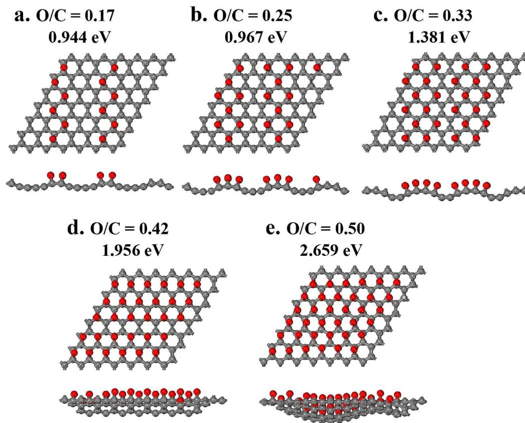
**Figure 8.** Molecular structures with an increasing concentration of epoxide function groups on a graphene surface and their band gap energies obtained with quantum chemical calculations: top view (image above) and side view (image below).
