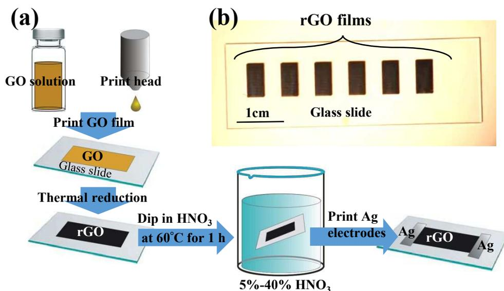
**Figure 1.** (a) Illustration of experimental procedures to fabricate inkjet-printed and HNO<sub>3</sub>-treated rGO films and (b) optical image of rGO films.
