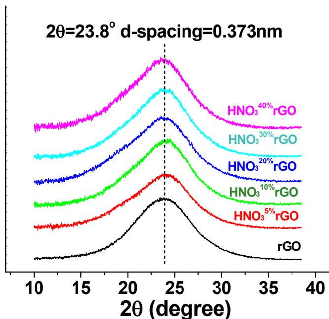
**Figure 6.** XRD patterns of the initial and HNO<sub>3</sub>-treated rGO materials.
