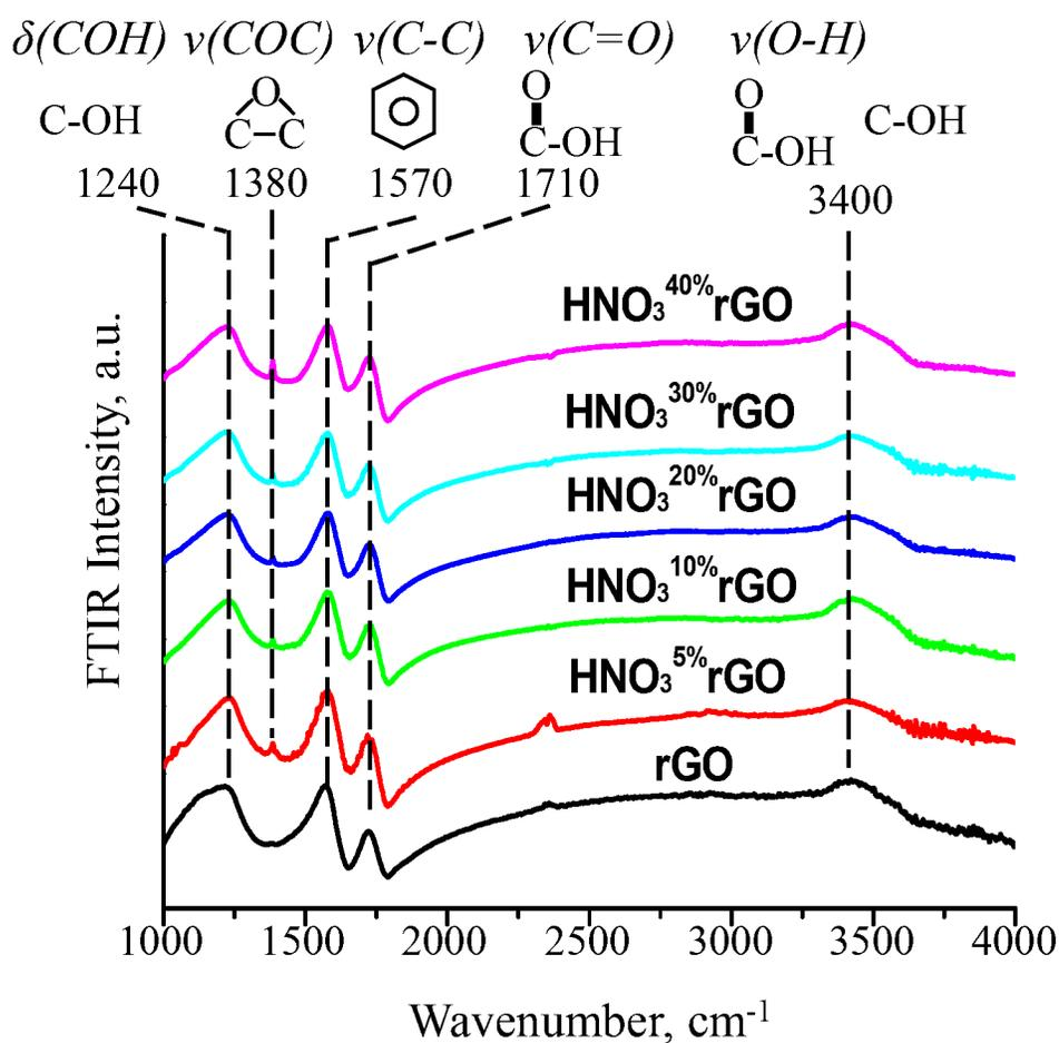
**Figure 4.** FTIR spectra of the initial and  $\text{HNO}_3$ -treated rGO materials.
