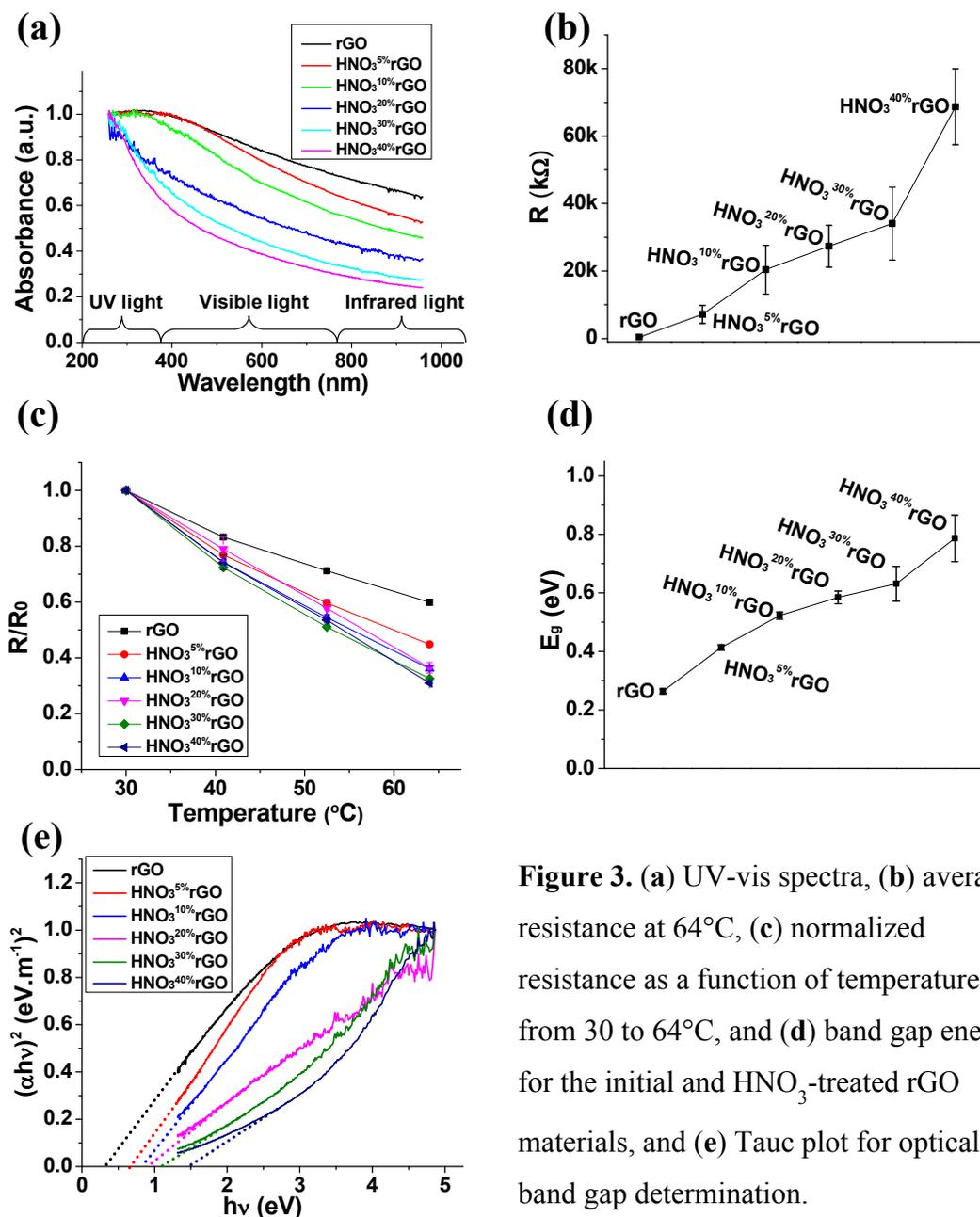
**Figure 3.** (a) UV-vis spectra, (b) average resistance at 64 $^{\circ}\text{C}$ , (c) normalized resistance as a function of temperature from 30 to 64 $^{\circ}\text{C}$ , and (d) band gap energy for the initial and  $\text{HNO}_3$ -treated rGO materials, and (e) Tauc plot for optical band gap determination.
