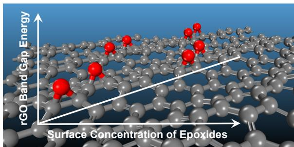
Functionalization of reduced graphene oxide with epoxide groups allows tuning its band gap energy
