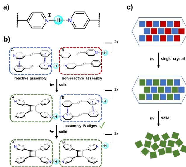
**Scheme 1** (a) N<sup>+</sup>-H<sup>+</sup>⋯N hydrogen bond. (b) Regiocontrolled cascade-like [2+2] photodimerization of 4-stilbazole. (c) Cascade transformation process (blue: photoactive assemblies; red: photostable assemblies; green: cyclobutane products).
