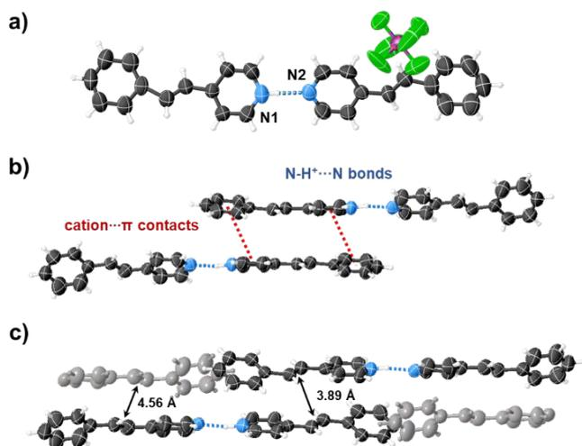
Fig. 1 Crystal structure [4-stilbz·(4-stilbzH<sup>+</sup>)(PF<sub>6</sub><sup>-</sup>)]. ORTEP views of (a) two-component dimeric array, (b) four-component assembly, (c) stacking of four-component assemblies.
