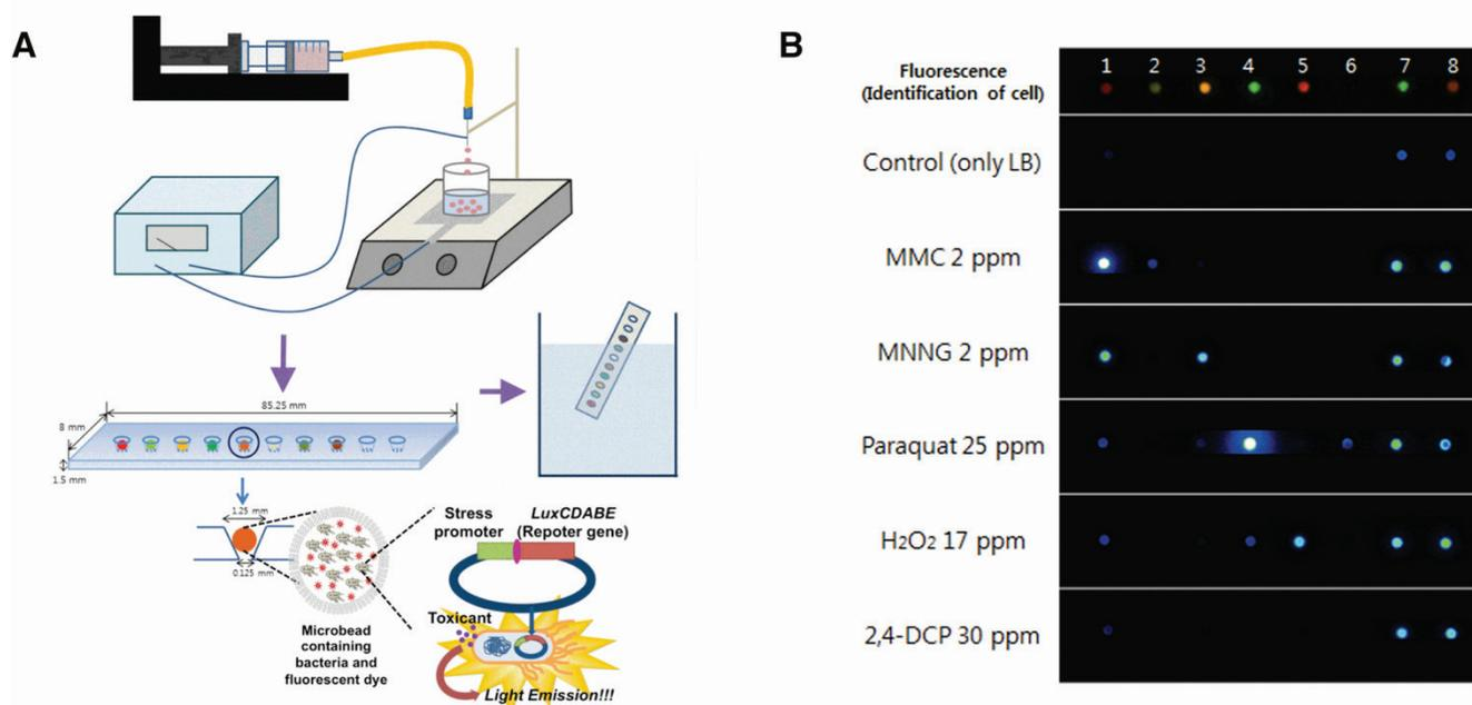
**Fig 4.** Dip-stick type biosensor for the detection of toxicants in water. (A) Schematic representation shows the process of building a dip-stick biosensor that contains genetically engineered bioluminescent bacteria for the detection of multiple pollutants. (B) Dip-stick biosensor bioluminescent response to five different model chemicals. Adapted with permission from ref. (147). Copyright (2014) Royal Society of Chemistry.
