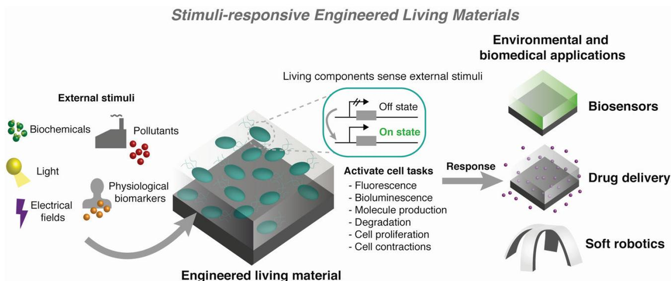
**Fig. 1** Stimuli-responsive engineered living materials. Schematic representation of an ELM that sense the external environment and respond in a controlled manner. Materials that contain genetically engineered living components are capable of sensing specific stimuli. Upon detection, cells can mediate a broad range of ELM responses. These include practical environmental and biomedical applications, such as biosensing, drug delivery, and robotic function.
