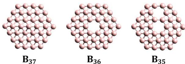
**Figure 1.** Three typical boron nanoflakes calculated to be stable<sup>10</sup>. The transmission and electronic properties of these structures and their isomers are investigated.
