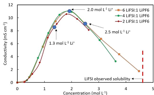
**Fig. 1.** Ionic conductivity as a function of total  $\text{Li}^+$  concentration for molar ratios of LiFSI: $\text{LiPF}_6$  salt added of 6:1 (orange squares), 4:1 (green circles), and 2:1 (red diamonds). Lines added to guide the eye. The three LiFSI-based electrolytes used in this study are indicated at the blue circle locations. The observed solubility for LiFSI is noted at the concentration where there is a vertical red dashed line.
