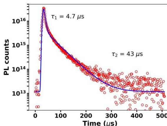
Figure 1. Time-resolved PL decay of the m-MTDATA/3TPYMB blend (red circles) shows prompt and delayed emission with time constants of 4.7  $\mu$ s and 43  $\mu$ s. A bi-exponential function convolved with experimental IRF is fit to the data and shown in blue.
