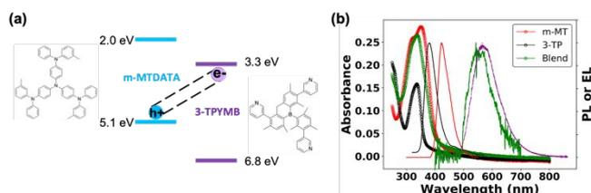
Figure 2. (a) State energies<sup>31</sup> and molecular structures of m-MTDATA and 3TPYMB. (b) Absorption (–o–) and PL spectra (–) of neat donor (red), acceptor (black) and blend films/devices (green) overlaid with EL spectrum (purple) of the blend device. The PL spectrum of the blend was measured from the solar cell device stack.
