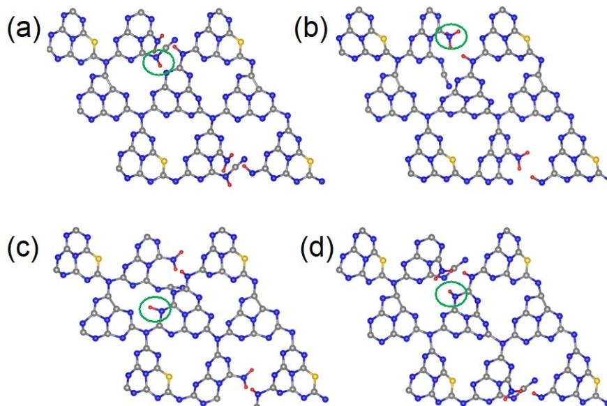
**Figure 1.** Optimized structures of dual defect ON-GCN tautomers. The structures are labeled based on the position of the circled hydrogen atoms as **(a)** NH-CN (most stable structure), **(b)** NH<sub>3</sub>, **(c)** N<sub>Hβ</sub> and **(d)** N<sub>Hα</sub> (least stable structure), Table 1. C: grey, N: blue, O: golden and H: red.
