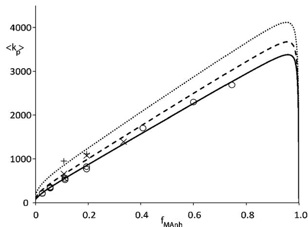
**Fig. 2** Average propagation rate coefficient ( $\langle k_p \rangle$ ) as a function of fraction MAnh in STY–MAnh copolymerization ( $f_{\text{MAnh}}$ ) at 25 °C ( $\circ$ ), 35 °C ( $\times$ ) and 50 °C ( $+$ ). Curves are calculated on the basis of the PUM and parameters from Table 1 (solid curve: 25 °C, dashed curve: 35 °C, dotted curve: 50 °C).<sup>5,10</sup>
