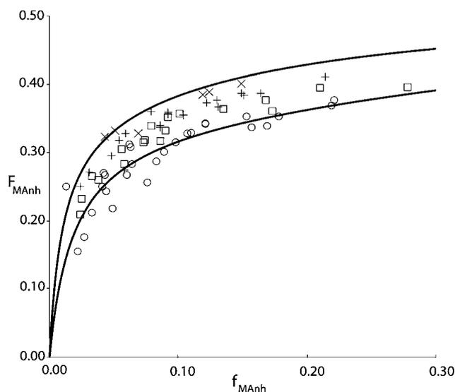
**Fig. 1** STY–MAnh copolymer composition ( $F_{\text{MAnh}}$ ) *versus* monomer feed composition ( $f_{\text{MAnh}}$ ) data from experiments in a CSTR at 60 °C ( $\times$ ), 90 °C ( $+$ ), 110 °C ( $\square$ ) and 140 °C ( $\circ$ ). Drawn curves are based on the penultimate unit model according to parameters shown in Table 1, at 60 °C (top curve) and 140 °C (bottom curve).<sup>10</sup>
