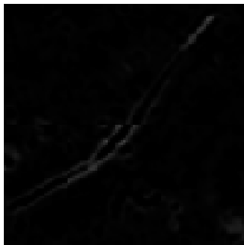
Fig. 8 Hyperspectral images composed of hyperspectral tiles that were collected using our in-house SPERO microscope. The image reveals a lack of harmony at the junction where the two hyperspectral tiles are joined. The horizontal midline of the images marks the location where the hyperspectral tiles meet.
