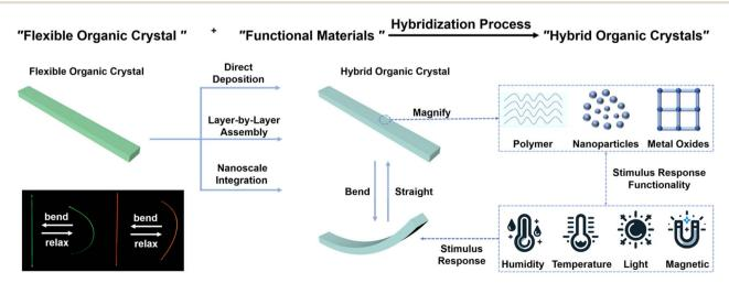
Fig. 3 Preparation process, deposition method, classification, functionality, and other details pertinent to the hybrid organic-polymer materials.
