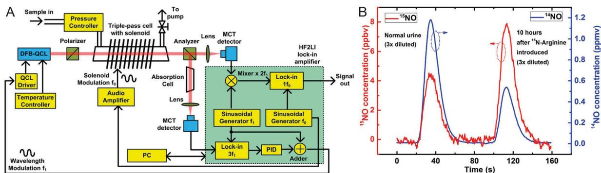
Fig. 3 (A) Schematic configuration of a FRS system. (B) Measurement of <sup>15</sup>NO (red) and <sup>14</sup>NO (blue) concentration after chemical conversion of nitrite/nitrate from patient's urine samples obtained before and after <sup>15</sup>N labeled arginine was introduced. Reproduced from ref. 132 with permission from Nature Publishing Group, copyright 2015.
