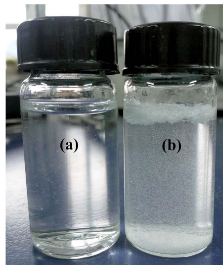
Fig. 7 The IBU solubilized by \beta -CDP (a) and its control group without the addition of \beta -CDP (b).
