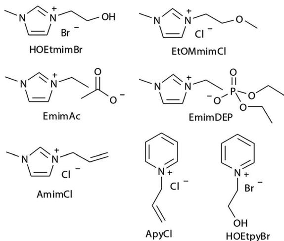
Fig. 7 The selected 7 ILs predicted by Liu *et al.* using COSMO-RS.<sup>78</sup> Reproduced from ref. 78 with permission from the Royal Society of Chemistry.
