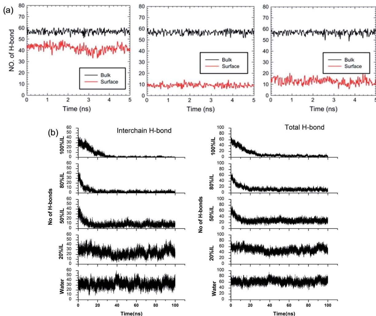
Fig. 12 (a) The change of H-bonds inside the cellulose layer (black) and at the surface (red). From left to right is [Bmim][PF<sub>6</sub>], [Bmim][OAc] and H<sub>2</sub>O.<sup>94</sup> (b) Effect of [C<sub>2</sub>mim][OAc]–water mixtures on the disruption of the inter-chain H-bonds and total H-bonds between cellulose at 160 °C.<sup>42</sup> Reproduced from ref. 42 and 94 with permission from Elsevier and the Royal Society of Chemistry.
