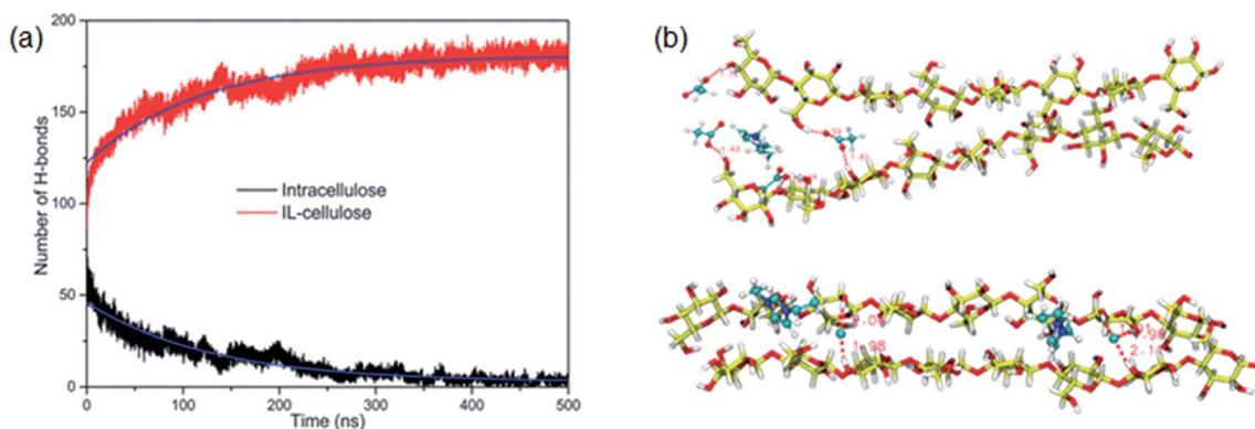
Fig. 13 (a) The change of intracellulose and cellulose–IL H-bonds during the simulation of a cellulose bunch in [Emim][OAc]. (b) Snapshots of H-bond formation between cellulose chains and ILs.<sup>105</sup> Reproduced from ref. 105 with permission from the PCCP Owner Societies.
