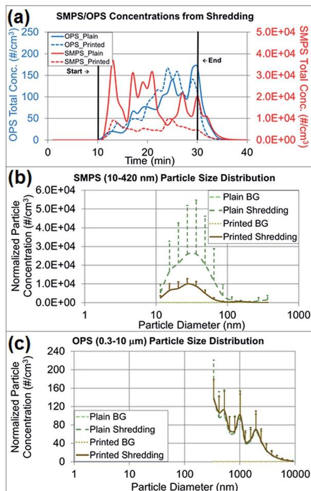
Fig. 6 RTI [OPS (0.3–10  $\mu\text{m}$ ) and NanoScan SMPS (10–420 nm)] data for shredding 40 sheets of plain and printed paper. (a) Area total particle concentration, as measured by RTIs. (b) Paper particle size distribution with standard deviations, as determined by NanoScan SMPS. (c) Paper particle size distribution with standard deviations, as determined by OPS.
