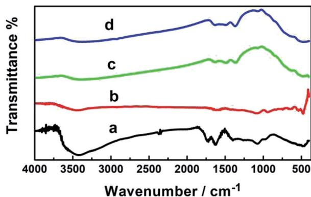
Fig. 4 FT-IR spectra of (a) GO, (b) GO-Ag, (c) GO-Ag-TiO<sub>2</sub>@ZnO, and (d) GO-TiO<sub>2</sub>@ZnO.
