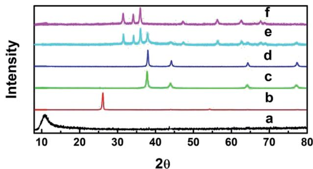
Fig. 1 XRD patterns of (a) GO, (b) graphite, (c) Ag, (d) GO-Ag, (e) GO-TiO<sub>2</sub>@ZnO, and (f) GO-Ag-TiO<sub>2</sub>@ZnO.
