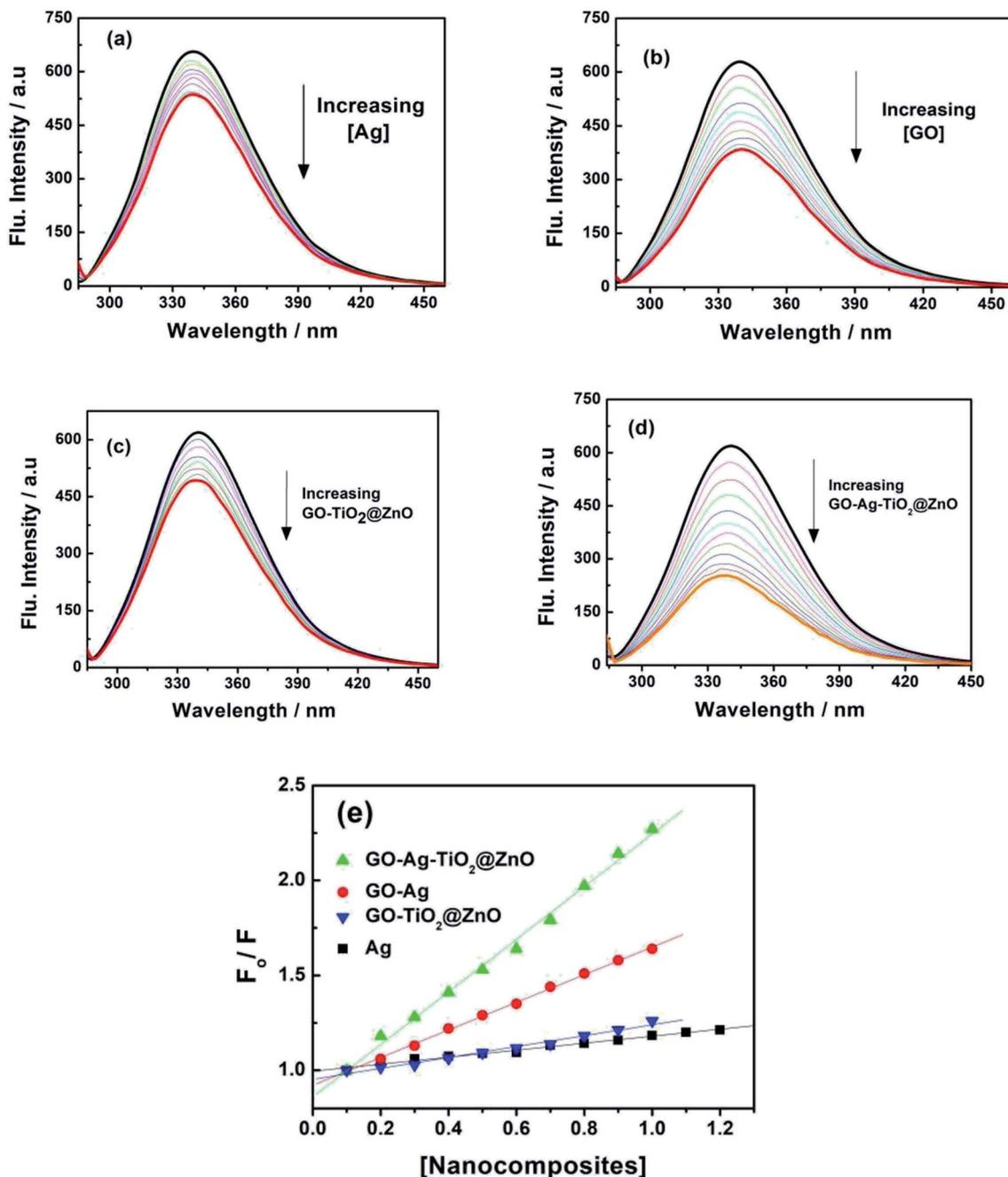
Fig. 7 Fluorescence spectra of BSA with different concentration of (a) Ag, (b) GO-Ag, (c) GO-TiO<sub>2</sub>@ZnO, and (d) GO-Ag-TiO<sub>2</sub>@ZnO at  $\lambda_{\text{ex}} = 280$  nm. (e) Stern-Volmer plots.
