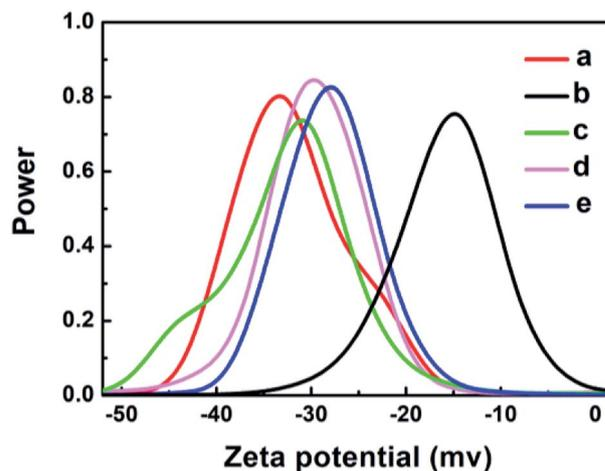
Fig. 3 Zeta potential graphs of: (a) GO, (b) Ag, (c) GO-Ag, (d) GO-TiO<sub>2</sub>@ZnO, and (e) GO-Ag-TiO<sub>2</sub>@ZnO in water.
