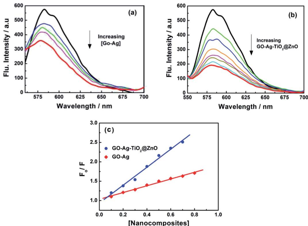
Fig. 8 Fluorescence quenching of ctDNA with different concentrations of (a) GO-Ag and (b) GO-Ag-TiO<sub>2</sub>@ZnO in Tris-HCl buffer;  $\lambda_{\text{ex}} = 260$  nm; (c) Stern-Volmer plots.
