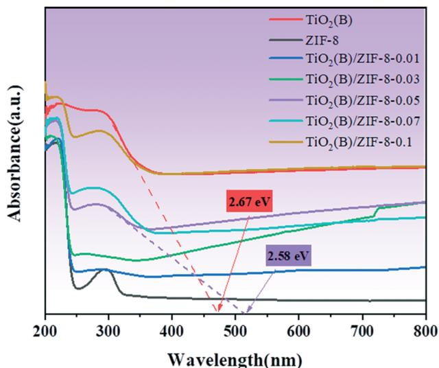
Fig. 5 UV-vis diffuse reflectance spectra of different samples.
