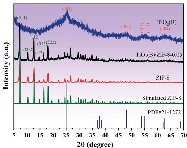
Fig. 1 XRD patterns of TiO<sub>2</sub>(B), ZIF-8, and TiO<sub>2</sub>(B)/ZIF-8.
