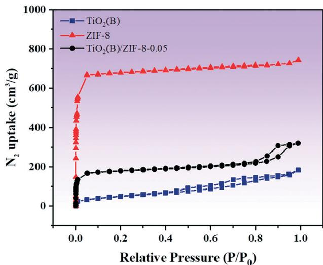
Fig. 4  $N_2$  adsorption isotherms measured at 77 K.
