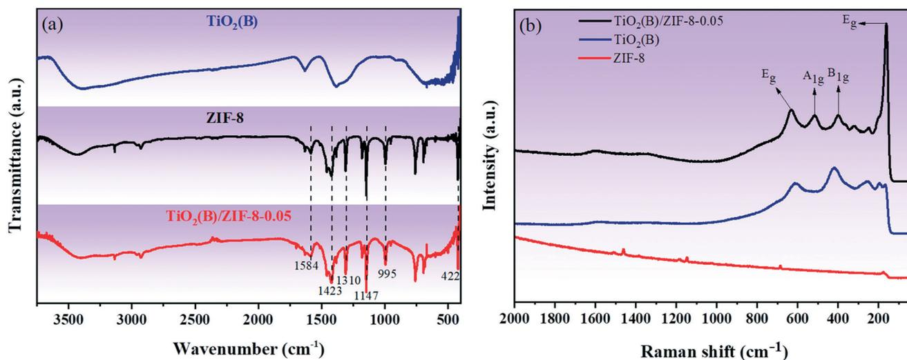
Fig. 3 (a) FT-IR spectra of  $\text{TiO}_2(\text{B})$ ,  $\text{TiO}_2(\text{B})/\text{ZIF-8}$  and ZIF-8; (b) characteristic Raman spectra of  $\text{TiO}_2(\text{B})$ , ZIF-8 and  $\text{TiO}_2(\text{B})/\text{ZIF-8}$ .
