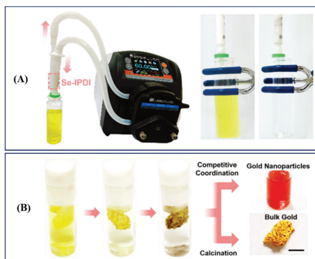
Fig. 11 (A) The equipment for simulating the dynamic extraction process in industrial treatment and the color change of the \text{Au}^{3+} solution before and after treatment with the system; (B) procedure of gold extraction with Se-foam and posttreatments by competitive coordination or calcination. Reproduced with permission from ref. 216. Copyright 2020 WILEY-VCH Verlag GmbH & Co. KGaA, Weinheim.
