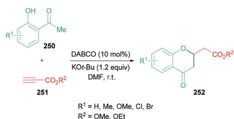
Scheme 64 DABCO-catalyzed synthesis of 2-alkyl-substituted chromanones from ortho -acylphenols and terminal alkynoates.
