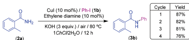
Scheme 3 CuI-catalyzed Goldberg type C–N coupling between iodobenzene ( 1b ) and 2-methylbenzamide ( 2a ) under air and at 80 °C in the eutectic mixture 1ChCl/2H 2 O: recycling studies.
