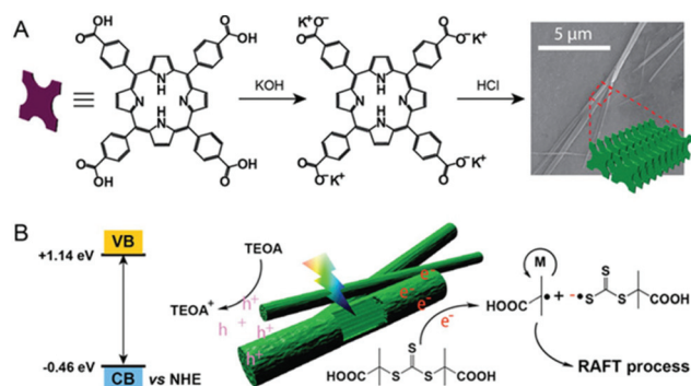
Fig. 15 Self-assembly of rod-like SA-TCPP and its use in PET-RAFT polymerization. Reproduced from ref. 153 with permission from Wiley-VCH Verlag GmbH & Co. KGaA, Weinheim, copyright 2020.
