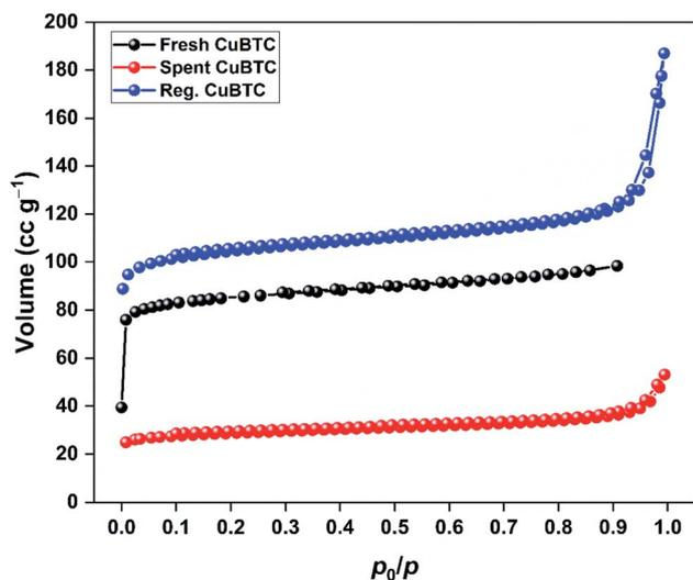
Fig. 9  $N_2$  adsorption-desorption isotherms of fresh, spent, and regenerated CuBTC.
