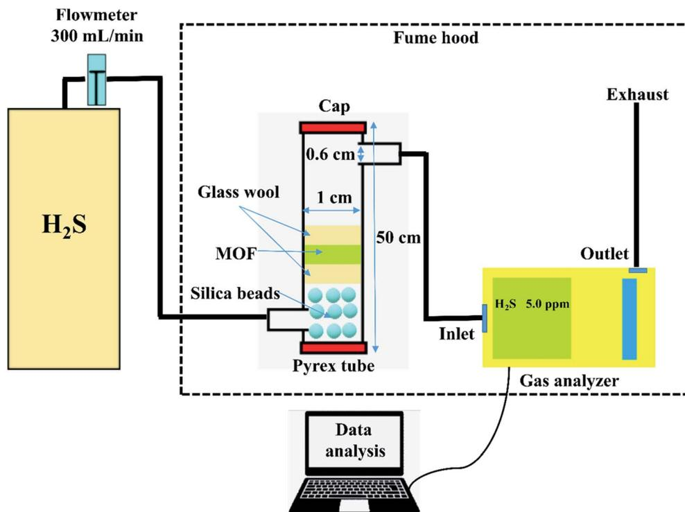
Fig. 1 Schematic illustration of the  $\text{H}_2\text{S}$  adsorption system.
