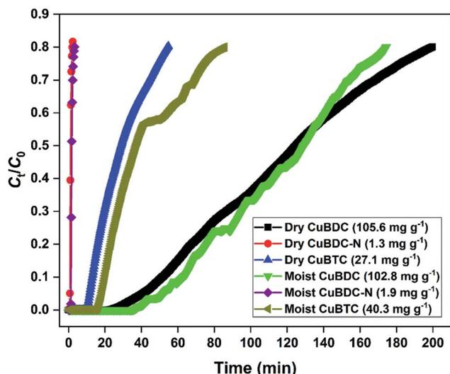
**Fig. 6** H<sub>2</sub>S breakthrough curve of dry and moist Cu-MOFs.
