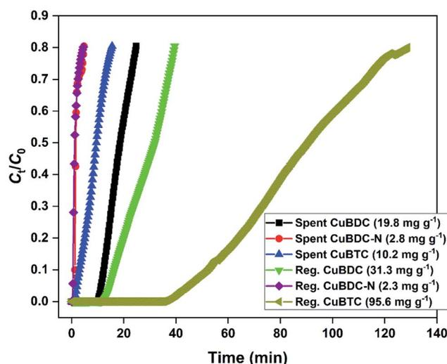
**Fig. 7** H<sub>2</sub>S breakthrough curve of spent and regenerated Cu-MOFs in the second cycle.
