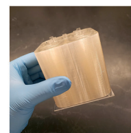
Fig. 1 Development of a mass-producible and deformation-free plastic spiral inertial microfluidic device. (a) A schematic diagram representing the fabrication process of the conventional polydimethylsiloxane (PDMS) spiral device and its stacking process for high-throughput application. (b) A schematic diagram representing the channel deformation in the PDMS spiral device and its effects on the device operation and performance; the color represents the relative channel deformation. (c) A schematic diagram representing the fabrication process of the plastic device and its key advantages; the plastic spiral device was designed by compensating for the channel deformation in the PDMS spiral device.
