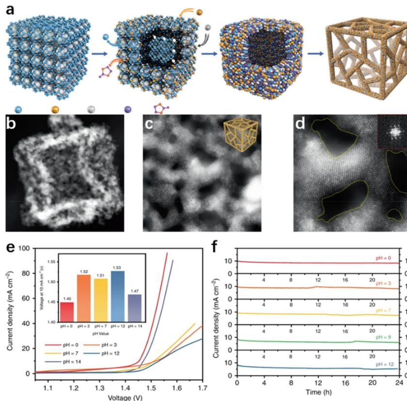
**Fig. 4** (a) The diagram of the synthetic process. The TEM (b) and HRTEM (d) images of RuIrO<sub>x</sub> nano-netcages, with a scale bar of 10, 5, and 2 nm. (e) The polarization curves and the voltages of RuIrO<sub>x</sub> nano-netcages at 10 mA cm<sup>-2</sup> (inset) throughout a wide pH range (0–14). (f) The current-time (*I*–*t*) curves of RuIrO<sub>x</sub> nano-netcages for 24 hours at various pH values.<sup>116</sup> Copyright 2019, Springer Nature.
