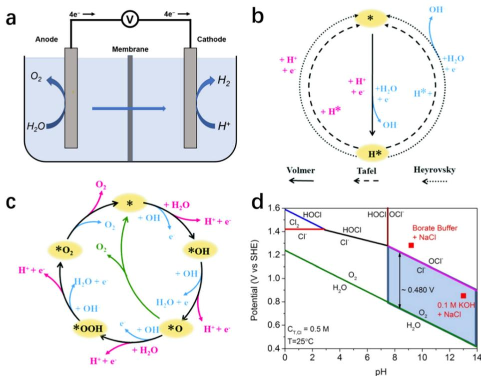
**Fig. 2** (a) Schematic illustration of electrochemical seawater splitting. Mechanism of HER (b) and OER (c) in alkaline (blue way) and acidic (pink way) solutions.<sup>54</sup> Copyright 2021, RSC. (d) A thermodynamically simulated Pourbaix diagram of saltwater containing oxygen and  $\text{Cl}^-$  redox reactions, with a total chlorine content of 0.5 M and a temperature of 25 °C.<sup>24</sup> Copyright 2016, Wiley-VCH Verlag GmbH.
