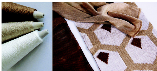
Fig. 30 (Left) Ioncell-F fibres produced using bleached pulp (white), cardboard (beige) and pulp with lignin as colorant additive (brown). (Right) Fabrics produced from the upcycled Ioncell-F fibres. Reproduced from ref. 264 with permission, copyright 2016 The Authors. Design: Marjaana Tanttu; photos: Eeva Suorlahti.
