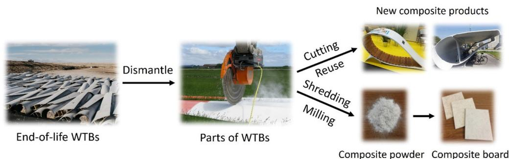
Fig. 4 Mechanical recycling processes of end-of-life WTBs.
