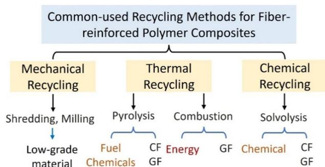
Fig. 3 Commonly-used recycling methods for fiber-reinforced polymer composites.
