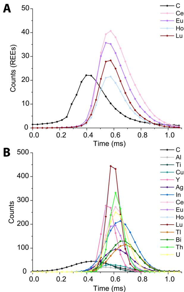
Fig. 6 Average time trace profiles for 1200 REE-doped polystyrene beads (A) and 2000 microdroplets containing 100 ng mL<sup>-1</sup> metals and 100 μg mL<sup>-1</sup> carbon (B) acquired with a time resolution of 36 μs.
