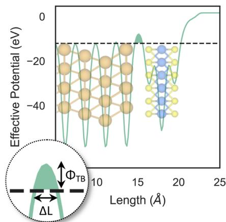
Fig. 6 Effective potential across the interface of the pristine Au/MoS<sub>2</sub> structure. The potential was projected in the direction of the interface. Highlighted in the figure are the tunnelling barrier height ( $\Phi_{\text{TB}}$ ) and the barrier width ( $\Delta L$ ).
