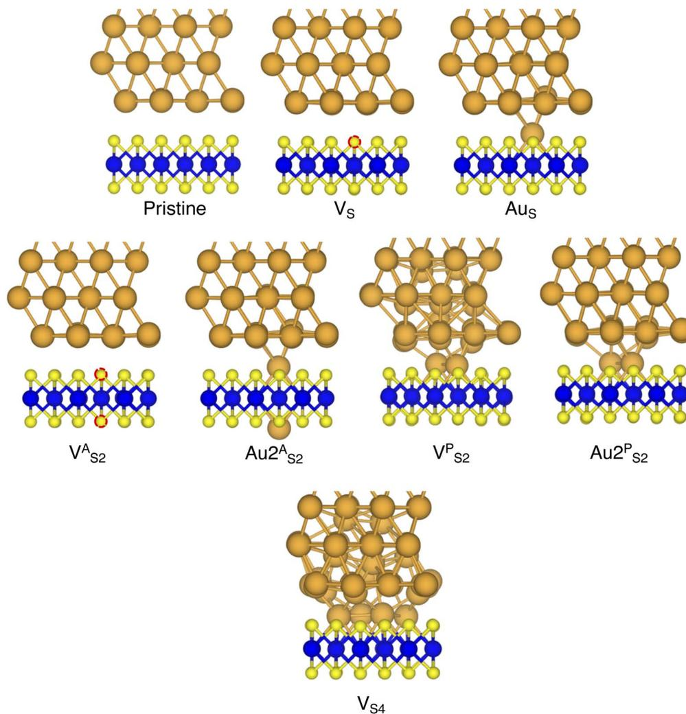
Fig. 2 Optimized geometries with DFT of selected Au/MoS<sub>2</sub> interfaces considered in this work. The pictures were taken in the vicinity of the contact area between the two materials. Interfaces V<sub>S2</sub><sup>A</sup> and V<sub>S4</sub> refer to MoS<sub>2</sub> with clusters of two and four S vacancies, although following geometry optimization such clusters were fully filled by Au atoms migrating from the above electrode.
