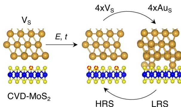
Fig. 8 Illustration of the proposed resistive switching mechanism and the possible Au/MoS<sub>2</sub> interfaces involved. Here, we propose the electric field ( $E$ ) and/or temperature ( $t$ ) as key quantities to generate extra S vacancies and to force the migration of Au atoms from (to) the metal electrode.
