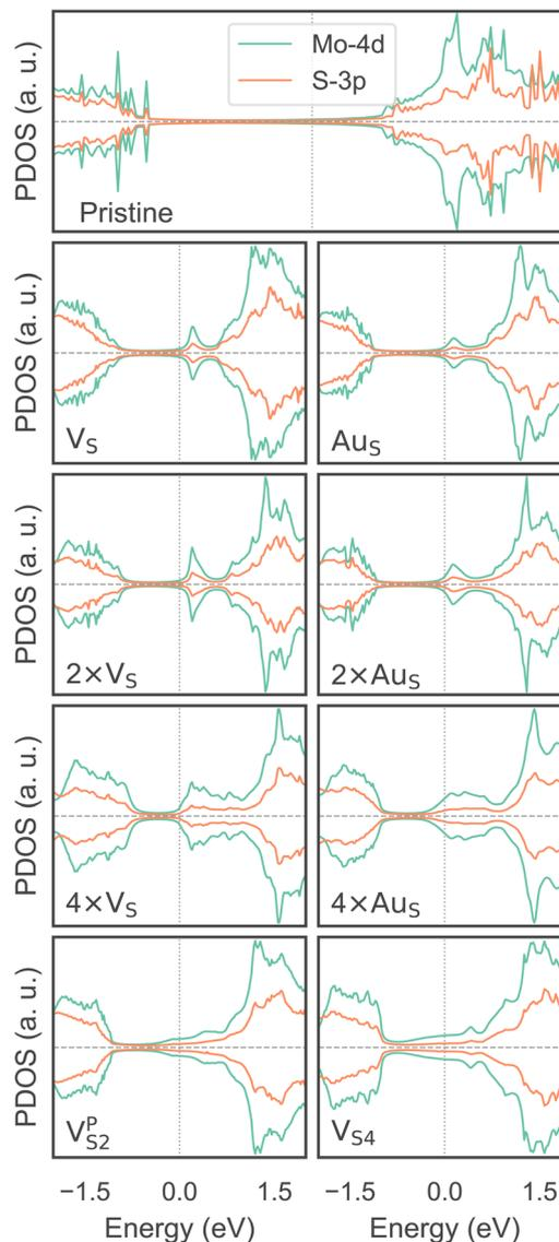
**Fig. 7** Density of states of selected interfaces, projected onto the Mo-4d and S-3p orbitals of MoS<sub>2</sub>. The plots, which result from the Green's function surface simulations, are centered around the Fermi level of each system (vertical dotted line).
