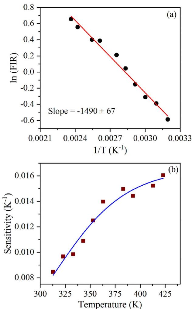
Fig. 8 UC-based ratiometric temperature sensing using  $\alpha\text{-NaYF}_4:\text{Yb}^{3+}/\text{Er}^{3+}$  nanophosphor: (a) plot of  $\ln(\text{FIR})$  (using 523 and 548 nm emission) as a function of the inverse absolute temperature, (b) temperature sensitivity as a function of temperature.
