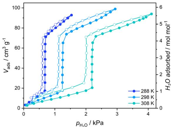
Fig. 3 Vapor adsorption isotherms of water recorded for **1** (**1**·**4H<sub>2</sub>O**) activated in a vacuum at 323 K. Full circles – adsorption, open circles – desorption.
