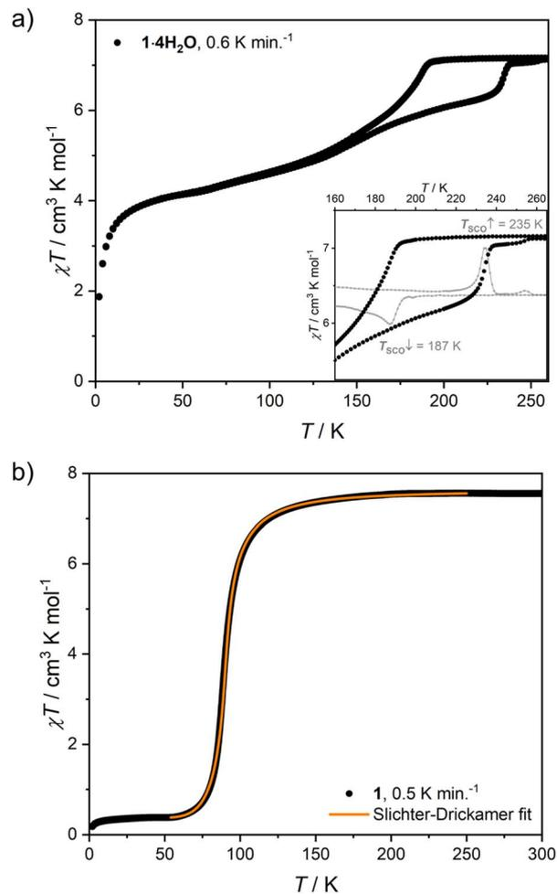
Fig. 4  $\chi T(T)$  dependence recorded for **1**·**4H<sub>2</sub>O** at  $\mu_0 H_{\text{dc}} = 0.1$  T (a) and close-up of the hysteresis loop with the corresponding  $d(\chi T)/dT$  derivative (inset).  $\chi T(T)$  dependence recorded for **1** at  $\mu_0 H_{\text{dc}} = 0.1$  T and the fit of the Slichter–Drickamer model (Eq. (2)) to the experimental data (b).
