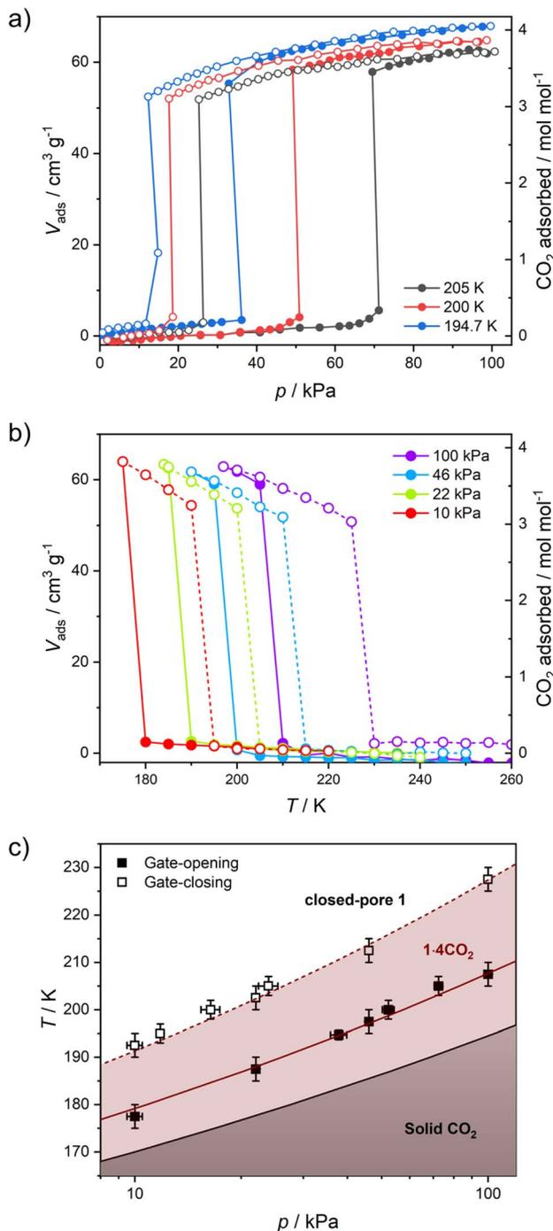
Fig. 5 CO<sub>2</sub> adsorption in **1** studied as isotherms at different temperatures (a) and isobars at different CO<sub>2</sub> pressures (b), and phase diagram of the  $1/\text{CO}_2/1 \cdot 4\text{CO}_2$  system based on these results (c).
