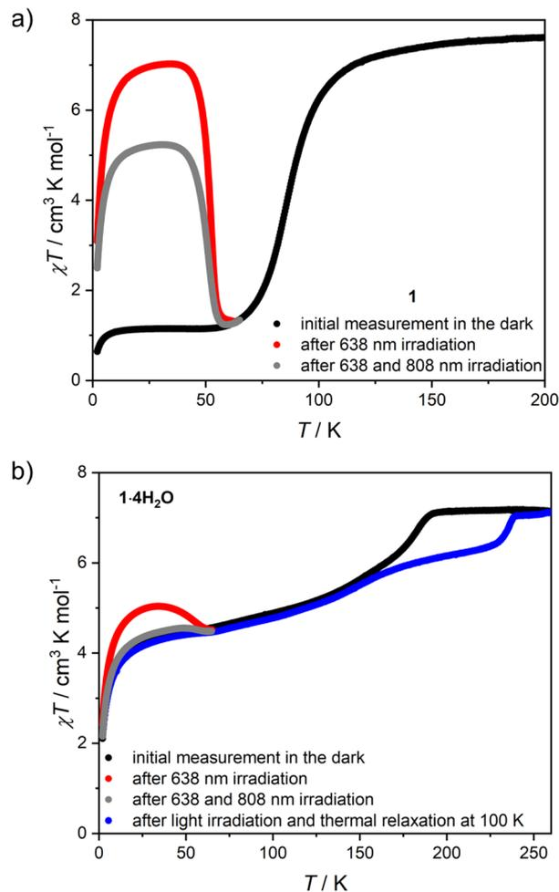
Fig. 7  $\chi T(T)$  variation recorded after 638 and 808 nm light irradiation for 1 (a) and 1·4H<sub>2</sub>O (b). Initial measurements and measurement after thermal relaxation were performed at 2 K min<sup>-1</sup> sweep rate, while measurements after light irradiation were performed at 0.3 K min<sup>-1</sup>.
